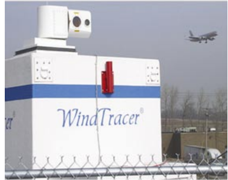
WindTracer profiles winds and detects windshear, turbulence, and aircraft wake vortices at both airports and onboard commercial airliners.
