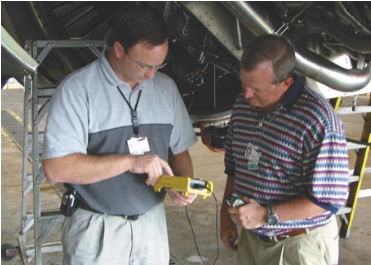
Delta Airline technicians Dane Swenson and Jim Elick use the Eclipse analyzer to test generator feeders on a Boeing 767 commercial aircraft.
