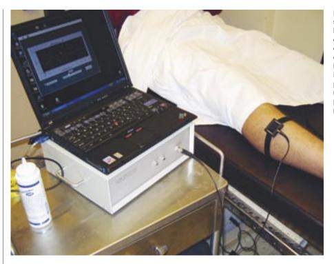
Luna's current compartment syndrome prototype is now being tested for noninvasive diagnosis. A next-generation design will reduce the size of the unit by a fourth and increase functionality. Here, its is shown taking internal pressure reading. The most common method for performing this test is a painful biopsy.
