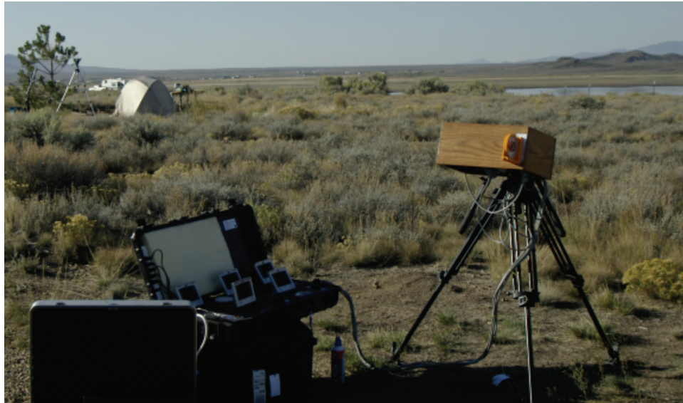
Figure 5. Mosaic camera array in position at Wild Horse Reservoir, NV. The reentry path was from far right (west) to the left in this view. Canadian VLF receiver and campsite is to the top left.
