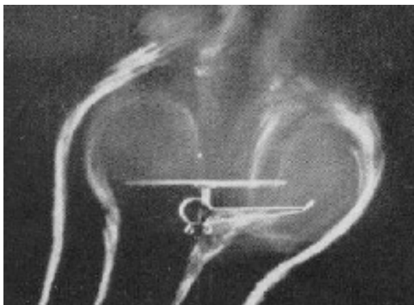
Figure 1. Smoke flow visualization of a rotor in vortex ring state (Drees, ref. 20).
