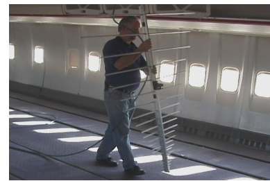
Figure 5. A log-periodic antenna simulating a portable transmitter
