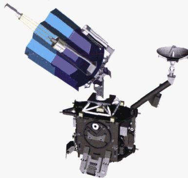
Figure 1. A possible application of the SPOT telescope architecture: a telescope mounted on the “top” (zenith) end of the Z1 truss
