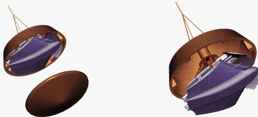
Figure 2. Extraction concept. Left illustration shows stowed airplane stowed inside the backshell just after heatshield release. Right illustration shows the extracted airplane prior to release from the AES.
