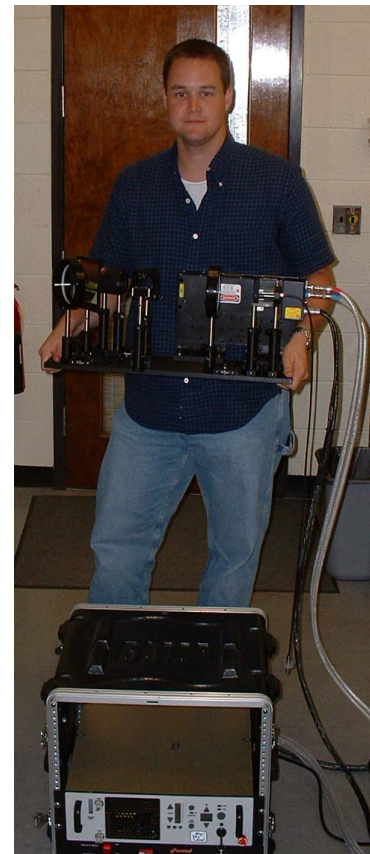
Figure 6.—Photographs of the prototype detector and instrument rack (which includes laser power supply).
