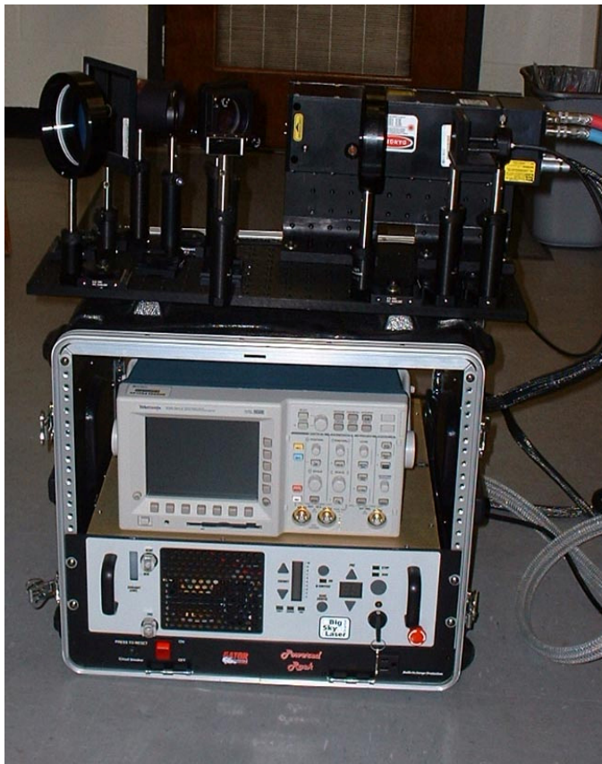
Figure 6.—Photographs of the prototype detector and instrument rack (which includes laser power supply).
