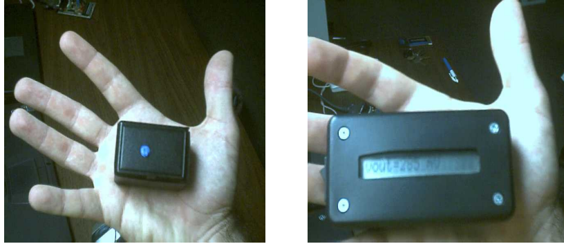
Figure 17. Photos of the remote wireless transmitter module (left) and the monitoring receiver module (right).
