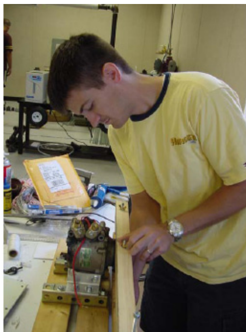
Figure 5.—(a) Scroll expander and (b) Scroll expander test set-up.
