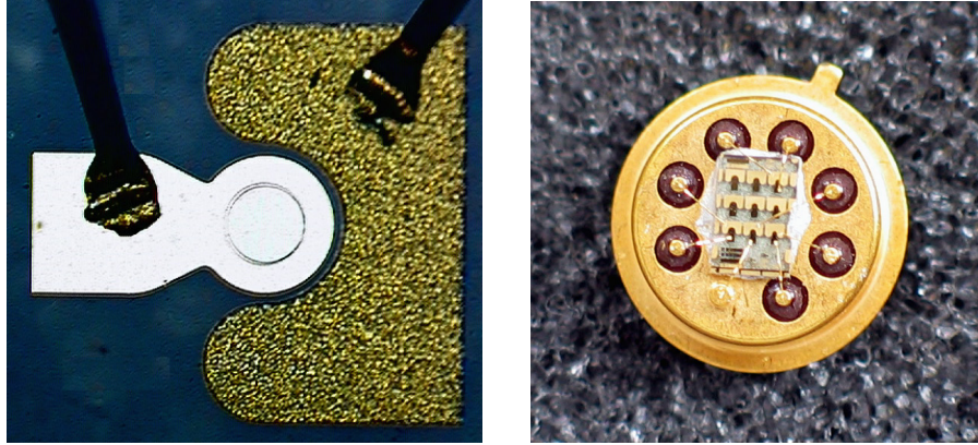
Figure 5.—AlGaIn/GaN Schottky diode hydrogen sensor (left) and the substrate mounted on a test fixture used for testing in chamber (right).
