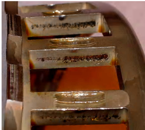
Figure 11.—Test 2 cage damage at test completion.
