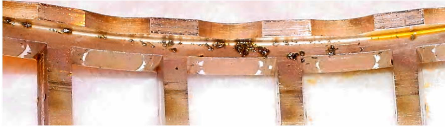
Figure 5.—Test 1 cage damage.
