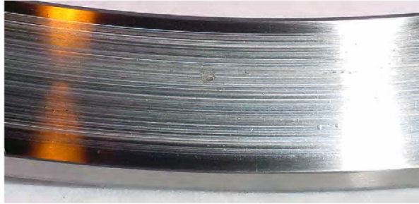
Figure 10.—Cup damage at test completion, observed after inspection 2, but did not progress.
