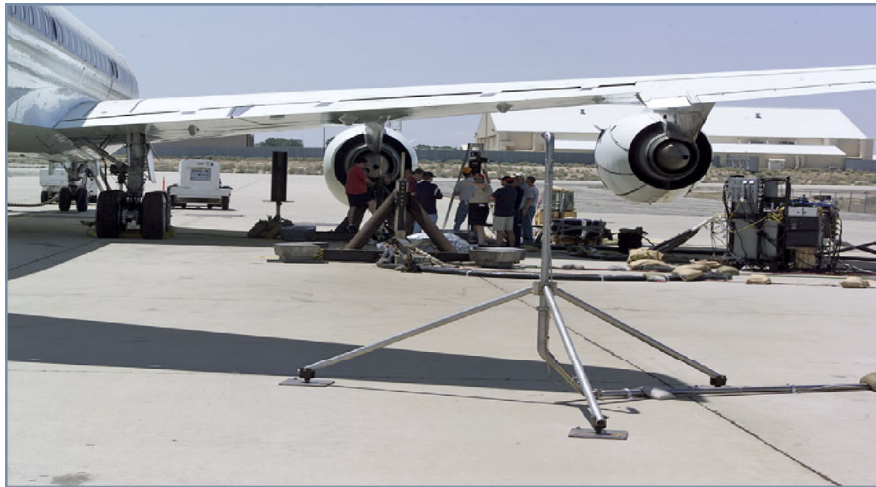
Figure 9.—Single sampling probe mounted on a tripod stand at 30 m.
