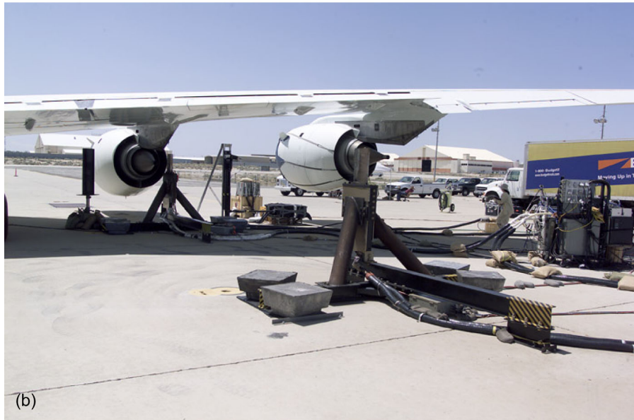
Figure C-1.—Experimental setup (a) Schematic of aircraft and 3 sample stands (red dots) at 1 m, 10 m, and 30 m downstream of the engine exit (b) Starboard side of NASA DC-8 aircraft with CFM56-2C1 engines, and 1 m and 10 m stands with multiple sample probes/lines connected to distribution box.
