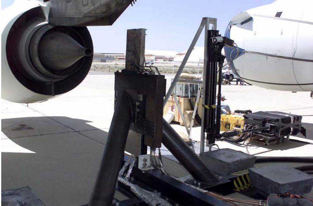
Figure K-3.—Photograph of CFM56-2 engine and sample rake at NASA APEX. All STAR measurements were taken at engine centerline, 1 meter from engine exit with water cooled sampling rake system. Thirty meter long sample lines to the STAR instrument were heated to approximately 90 °C.
