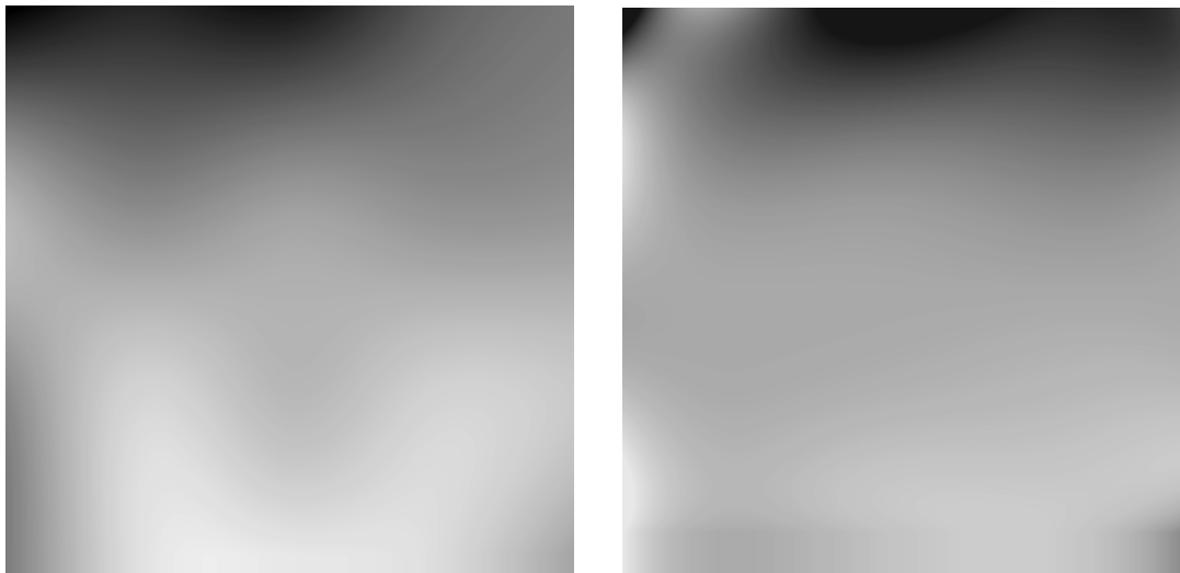
Figure 3: Adopted low order flat field images for the G230LB (left) and the G430L (right) are illustrated. The value of the G230LB I_{\text{flat}} ranges from 0.964 to 1.012, the G430L from 0.936 to 1.019, and the G750L (not shown) from 0.864 to 1.018.
