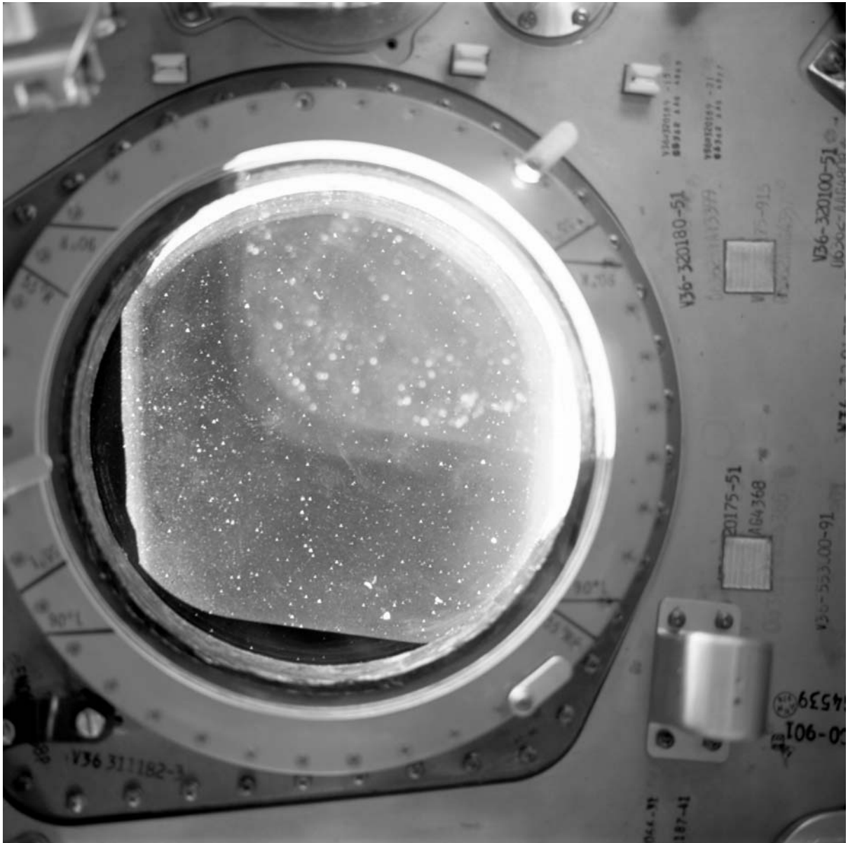
Photo 29. CM Hatch Window Contaminated During Apollo 9 Mission
