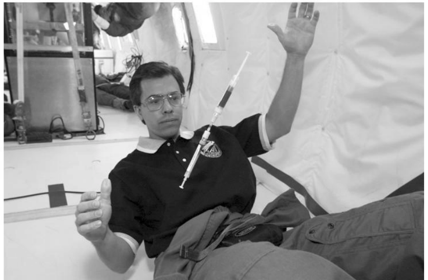
Figure 5. The Blood Collection/Preservation/Storage Apparatus designed to safely preserve of whole blood samples during microgravity conditions. Whole blood is collected into a Monovette containing anticoagulant, and is transferred to a Monovette containing preservative via a novel interlink adaptor. Use of this device is highly advantageous during field studies, as it greatly simplifies operations, reduces operator time and improves safety by nearly eliminating exposure to liquid blood samples. This device was validated during microgravity conditions onboard the NASA KC-135 parabolic flight aircraft in 2000. Top and upper right: BCPSA in use at Devon Island; right: BCPSA reduced gravity evaluation.
