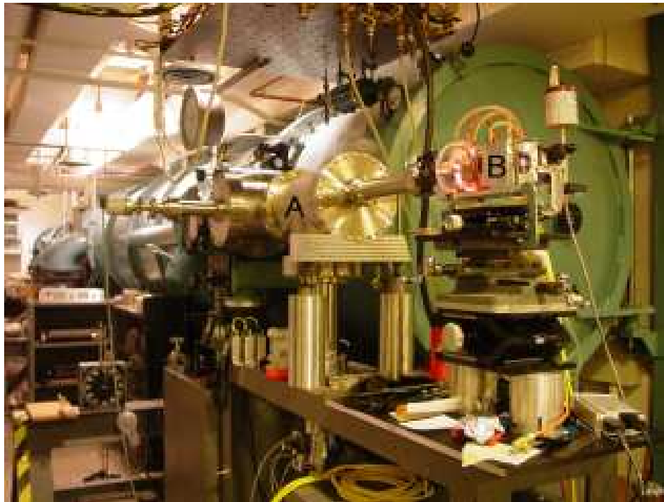
Fig. 1.— The 10.7-m normal-incidence vacuum spectrograph with foreoptics system.
