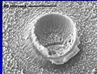
Impact Crater in FEP Teflon
