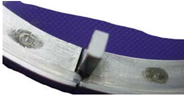
Backplate failure during test phase of advanced design misalignment tests
