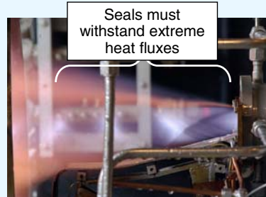
Baseline control surface seal design
