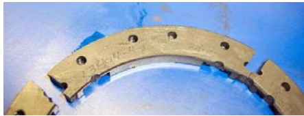
Back Ring Tab Failure
