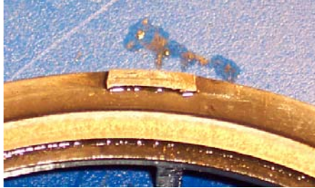
Backplate Tab Failure
