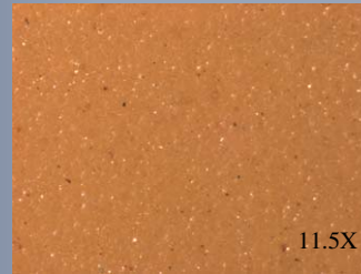
Optical micrograph of Esterline Kirkhill-TA XELA-SA-401.
