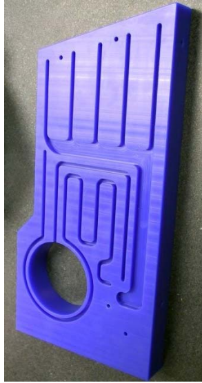
Wax model of sidewall showing cooling channels
