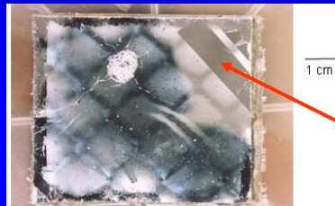
Tape Peeled Segment On Back of Array Showing Contaminant Removal
