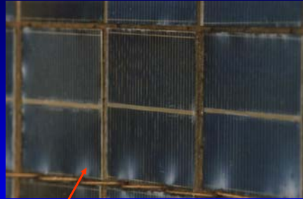
Oxidized Silicone Contamination on Front Side of MIR Array
