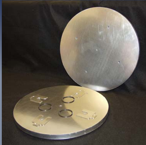
Photo of the Compression Set Fixture
