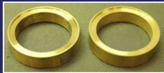
Seal surface pair after gold plating.
