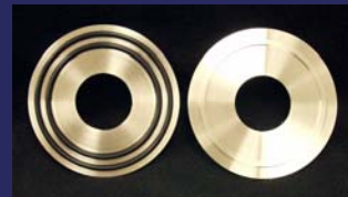
Photo of rigid metal interface concept test specimens
