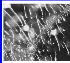
DC93-500 Exposed to 2.3e20 atoms/cm 2
