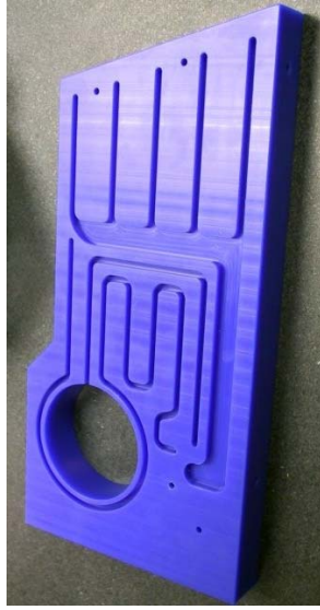
Wax model of sidewall showing cooling channels
