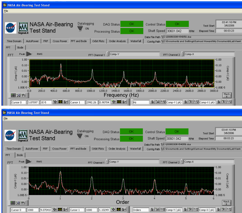
Figure 9.—FFT plots showing frequency and order components respectively at the compressor end of the rotor.
