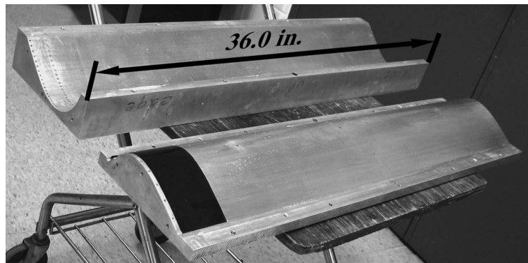
Figure 2.4. A CNC-machined aluminum mold was used to fabricate “PakB” blades (top: side view, bottom: top view).
