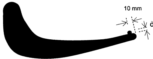
Figure 1.6. The “Langston” blade with a Gurney flap attached to the pressure surface near the trailing edge (from Byerley [6]).
