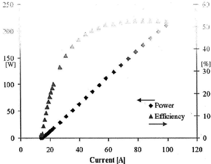
Figure 6 Typical L-I curve for LDA, from M. Stephen [2]
