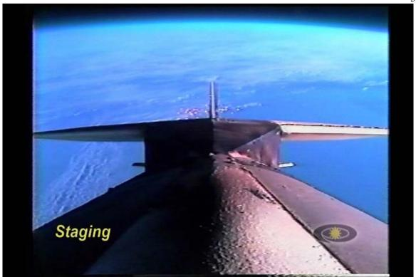
Figure 47. Tail-off +20 sec. Sporadic large particle emissions - which may continue for several hundred seconds.
