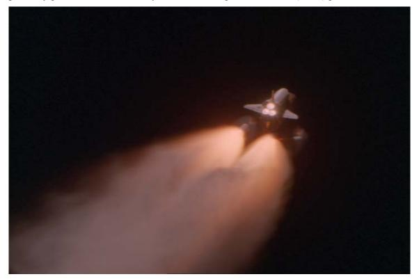
Figure 27. Separation +5 seconds; Chamber pressure < 6.9 kPa (< 1 psia). Tail-off ejecta are present but not yet resolved in the ground-based imagery due to limited dynamic range (blooming) in the image.
