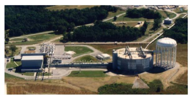
Figure 72. The J-6 Altitude Simulation Cell at AEDC is routinely used to test SRMs in a low pressure environment (1.38 kPa (<0.2 psia)) – effectively duplicating space vacuum conditions.
