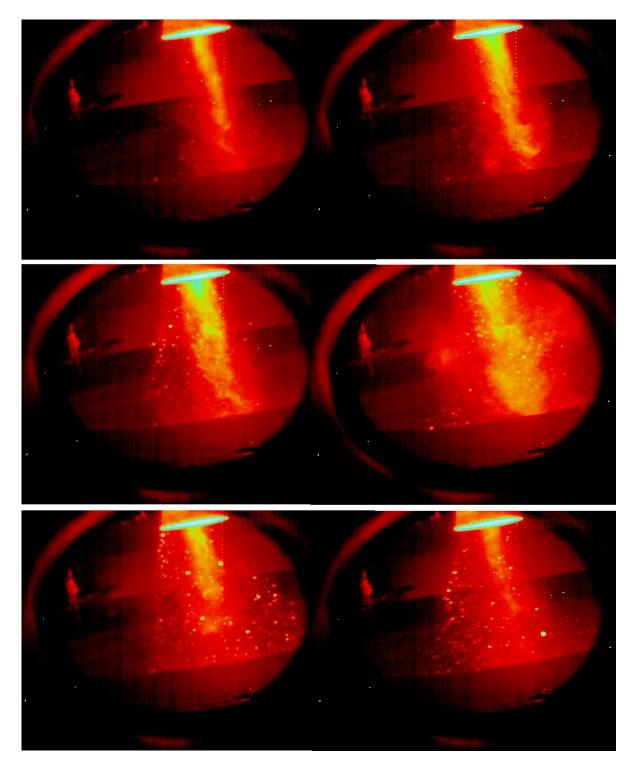
Figure 77. Star-37 SRM static spinning (60 rpm) vacuum test within the AEDC J-6 vacuum chamber. The sequence (read left to right and downward) illustrates a slag expulsion event approximately 6 seconds after the onset of Tail-off. (Chamber pressure < 6.9 kPa (< 1 psia)) (Frame Rate: 45 fps)
