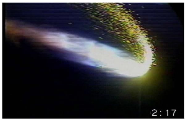
Figure 5. Dual Plumes. Pyrolysis gas and large (D>500  $\mu$ m) solid particulates are easily distinguished in this Tail-off image from an STS-103 in-situ camera. Differential atmospheric drag has separated the plumes according to area-to-mass ratios. During static ground testing, the two components are not visually differentiated.
