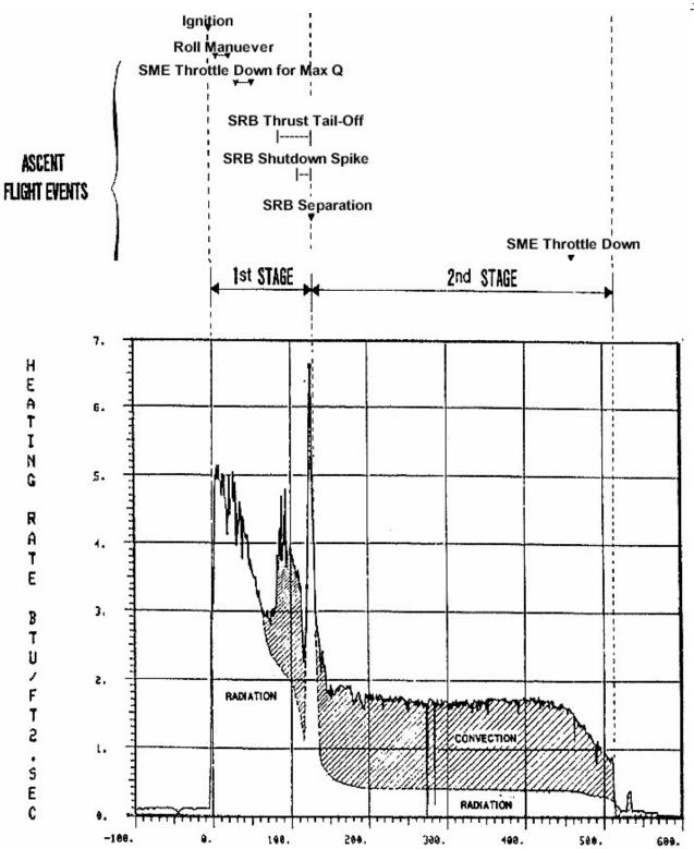
Figure 18. Typical Space Shuttle orbiter heat shield environment during flight. The radiative pulse at Tail-off is clearly evident at approximately 120 seconds into flight. (Greenwood et al., 1983).
