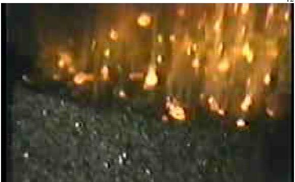
Figure 4. Image from high speed film of SRM burning propellant grain (19% Al, HTPB, AP). Agglomerates of approximately 50-500  $\mu$ m diameter are continuously liberated from the surface and then entrained in the flow exiting the nozzle. (United Technologies).
