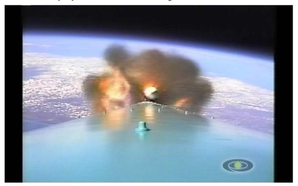
Figure 63. Tail-off phase of an air-lit Delta II booster. Large particulates are seen issuing from the SRM. Note the bright plume has contracted and darkened significantly relative to the previous frame – indicating that chamber pressures have declined into Tail-off.
