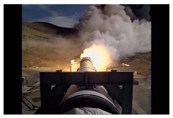
Figures 13. Optical imagery of Static SRB test (facing aft). Slag expulsion is not evident at Tail-off (lower frame). (Thiokol Photos).
