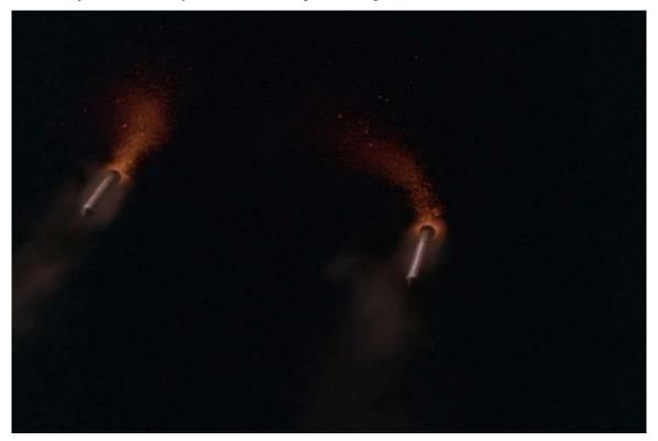
Figure 33. Separation +30.5 seconds. Chamber pressure < 6.9 kPa (< 1 psia). Numerous Tail-off ejecta are clearly resolved as the plume brightness fades. Ejecta continue to stream from the SRB, although at a reduced rate, for several minutes.
