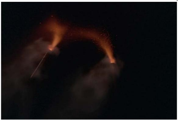
Figure 32. Separation +24.5 seconds. Chamber pressure < 6.9 kPa (< 1 psia). Numerous Tail-off ejecta are clearly resolved as the plume brightness continues to fade.
