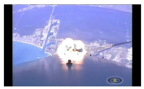
Figure 58. During the main phase of the booster burn, the plume is devoid of significant large particle content. Sporadic flashes are seen but these may be debris dislodged from the exterior surface. Figs. 58-61: April 7, 2001 Delta II Odyssey.
