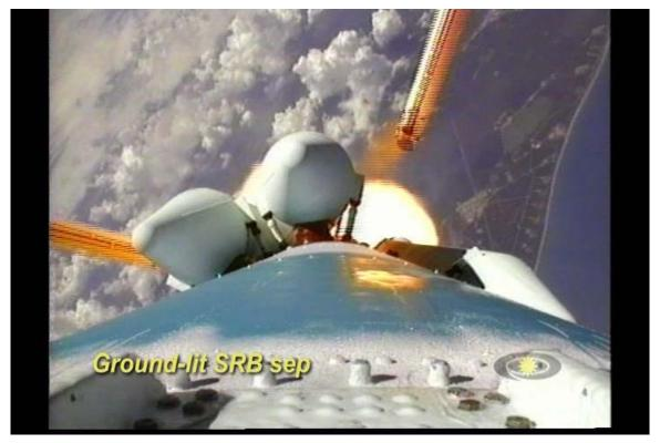
Figure 67. These Delta II booster are essentially completely depleted prior to separation. This may be why Tail-off emissions are sometimes more difficult to discern – the emissions are obscured by the main engine and the air-lit booster plumes.
