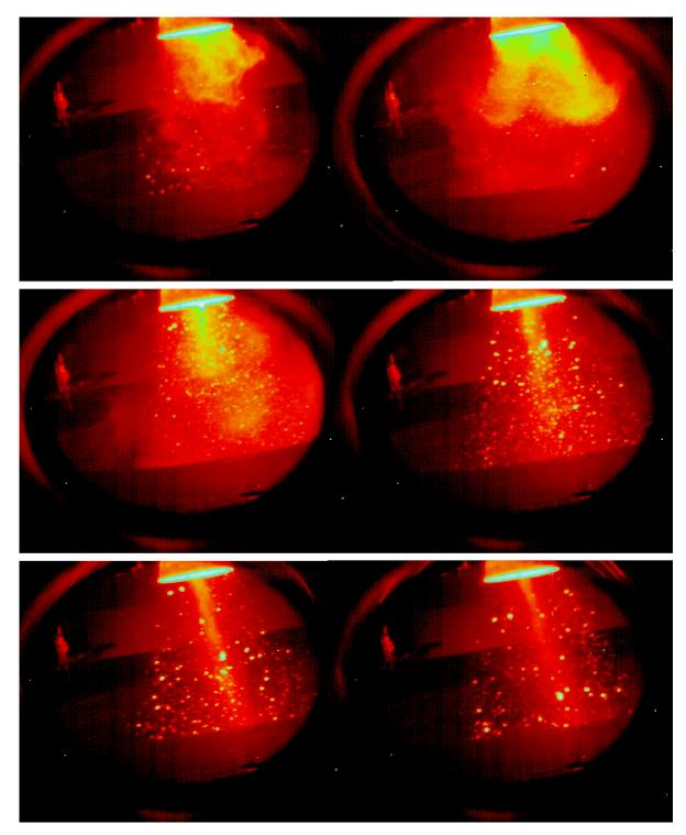
Figure 78. Star-37 SRM static spinning (60 rpm) vacuum test within the AEDC J-6 vacuum chamber. The sequence (read left to right and downward) illustrates a large slag expulsion event approximately 8 seconds after the onset of Tail-off. (Chamber pressure < 6.9 kPa (< 1 psia)) (Frame Rate: 45 fps)
