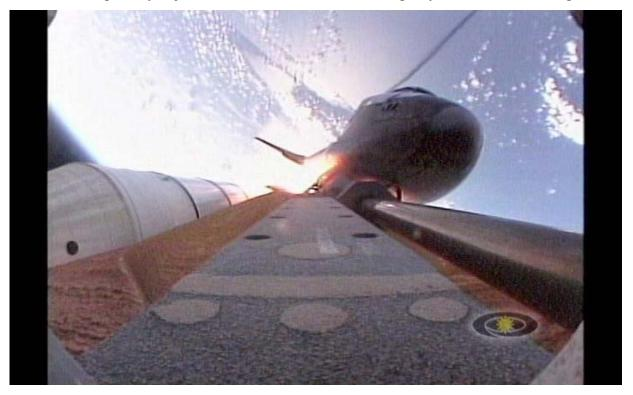
Figure 98. Space Shuttle Reurn-to-flight mission will have multiple camera enhancements (three per SRB with one aft pointed). (STS-112 Rocket Cam Image by Ecliptic Enterprises Inc.).
