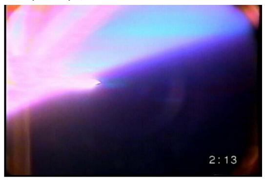
Figure 33. STS-101 Right SRB (as viewed from the Left SRB). Separation +9 seconds. (Chamber Pressure < 6.9 kPa (< 1 psia) for this and all subsequent images). Although the image is saturated (due to limited dynamic range and intense emissions), the two gaseous/dust and solid particulate plumes are distinctly visible.
