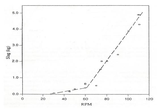
Figure 96. Slag deposition history or a Star-48 SRMs spinning at various rates. Agglomerates, that would otherwise escape through the nozzle during the main burn, are driven outward to the chamber walls by centrifugal force (e.g. 2 Gs for a 1 m diameter motor spinning at 60 rpm). At Tail-off, although more slag is ostensibly available for ejection, centrifugal effects may recapture many of the particulates leading to a net reduction of emissions. (Salita 1995)
