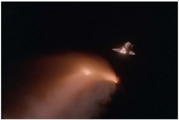
Figure 28. Separation +12 seconds; Chamber pressure < 6.9 kPa (< 1 psia). Tail-off larger ejecta are clearly visible, smaller objects are becoming visible at the plume perimeter.
