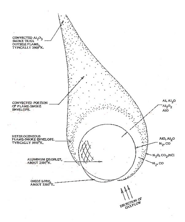
Figure 7. Detailed schematic of the morphology of a burning Aluminum Agglomerate. The oxide envelope, comprised of dust-like  $(0.1 < D < 100 \mu m)$  particles is continually swept away by the exhaust flow and exits the nozzle giving rise the plume's characteristic white color. The aluminum droplet is gradually consumed by oxidation unless it and its oxide cap (or lobe) are either trapped or escape intact as described in the text. (Price and Sigman 1994.)
