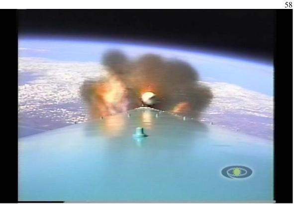
Figure 64. Tail-off phase continues for an air-lit Delta II booster. Large particulates issue from the SRM for several seconds prior to separation.
