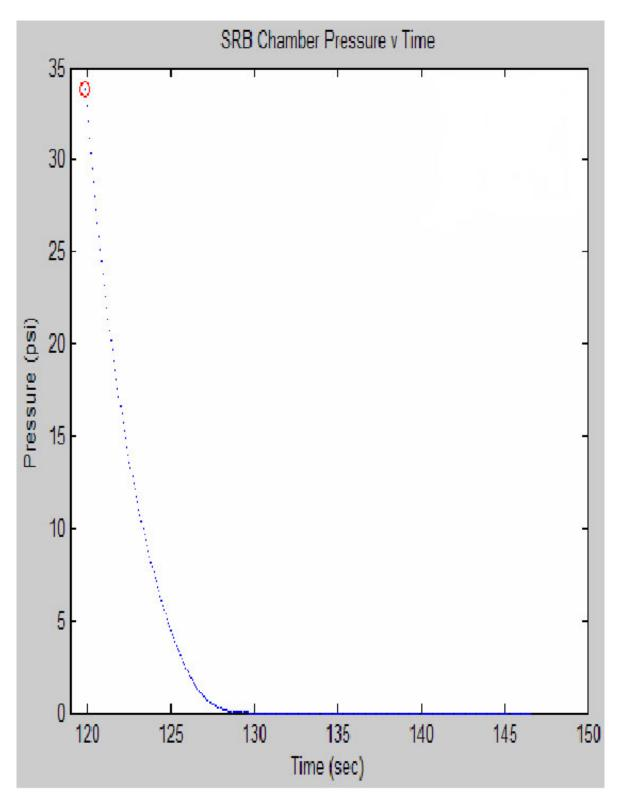
Figure 22. Extrapolated pressure profile for the P<241 kPa (<35 psia) regime. Correlating this figure with time-step imagery of SRB flight reveals that the mass of Tail-off ejection occurs at chamber pressures below 6.9 kPa (1 psia) – consistent with low-pressure boil-over.
