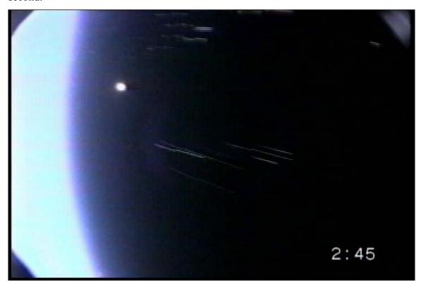
Figure 39. Separation +40.5 seconds. Emissions are ebbing but continue. These streaks are self-emissions from the descending Left SRB.
