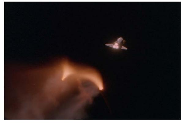
Figure 29. Separation +16.5 seconds; Chamber pressure < 6.9 kPa (< 1 psia). Smaller Tail-off ejecta visible as a mist that is on the cusp spatial resolvability.
