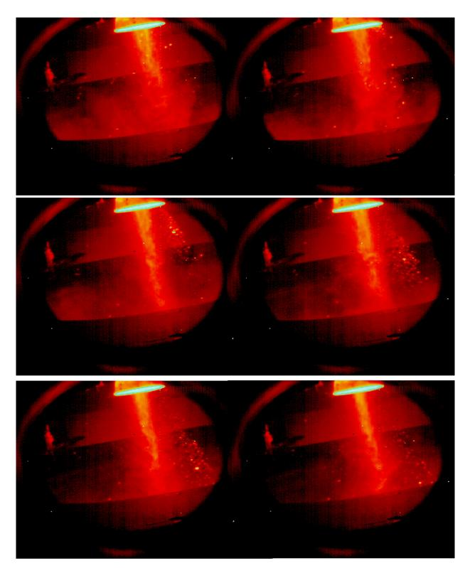
Figure 76. Star-37 SRM static spinning (60 rpm) vacuum test within the AEDC J-6 vacuum chamber. The sequence (read left to right and downward) illustrates a slag expulsion event during the beginning of Tail-off (4 seconds after onset; Chamber pressure < 6.9 kPa (< 1 psia). (Frame rate: 45 frames per second (fps))
