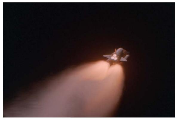
Figure 25. Separation Cue -0.0 second; Chamber pressure 6.9 kPa (10 psia). No Tail-off ejecta present, but shuttle base heating indicates some particulates are present in the plume.
