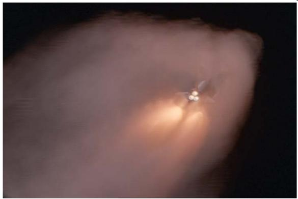
Figure 26. Separation + 1 second; Chamber pressure ~3.4 kPa (~5 psia). Tail-off ejecta are probably present but obscured by the Booster Separation Motor (BSM) plume.
