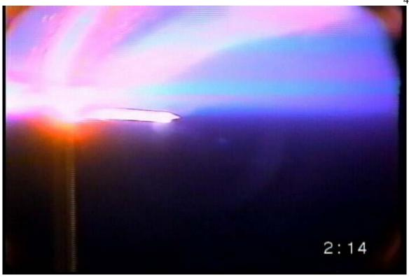
Figure 34. Separation +10 seconds. Solid particulates are visible in the solid particulate plume.
