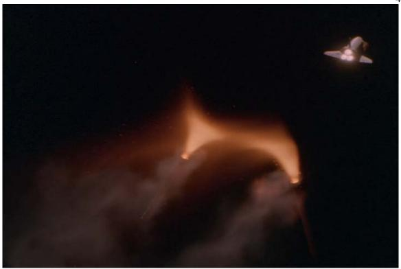
Figure 30. Separation +20.5 seconds; Chamber pressure < 6.9 kPa (< 1 psia). Smaller Tail-off ejecta are becoming more clearly differentiated and spatially resolved.
