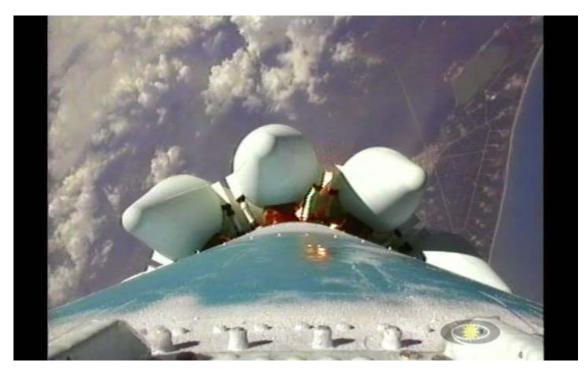
Figure 66. While the viewing angle and resolution are poor, there are brief large particulate emissions less than 1 second prior to booster separation in this June 6, 2003 Delta II Spirit launch (Figs 66-67). Note faint embers between two boosters at left center of photo.
