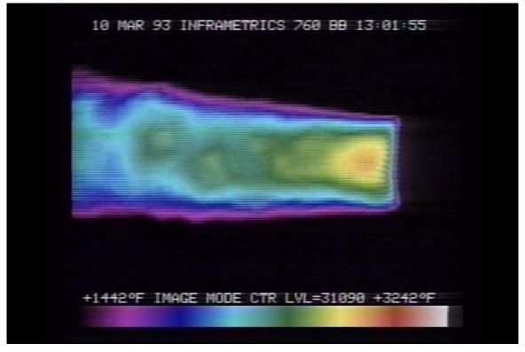
Figure 15. SRB Static test (non-vacuum) - beginning of Tail-off phase (ie. declining chamber pressure) revealed by turbulent flow and less expansive plume resulting in higher plume temp (~3000F). No solid particulates are discernable. (Thiokol photo).
