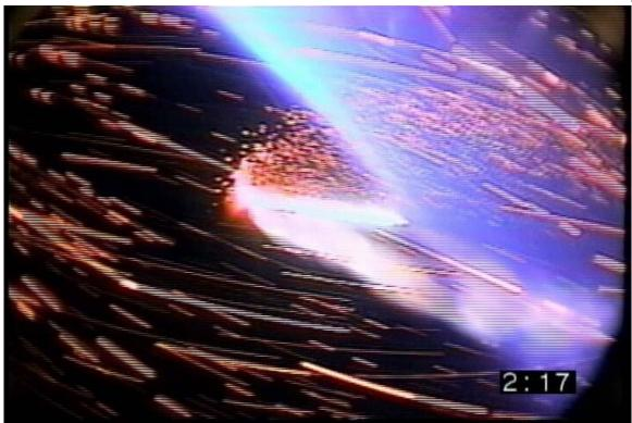
Figure 36. Separation +12.5 seconds. Self-emissions from the Left SRB occupy the foreground. In audio data, a solid metallic 'ping' is heard when these particles strike the SRB exterior – indicating the objects solidify quickly and thus have a high melting point (ie.  $Al_2O_3$ ).
