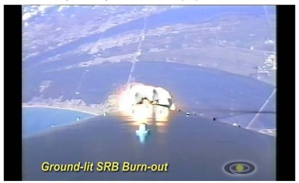
Figure 59. During the Tail-off phase large particles are clearly evident emanating from the SRM booster.
