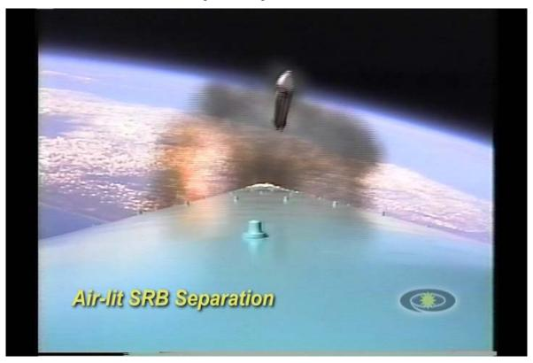
Figure 65. Delta II air-lit booster separation. Large particulate emissions are no longer discernable.
