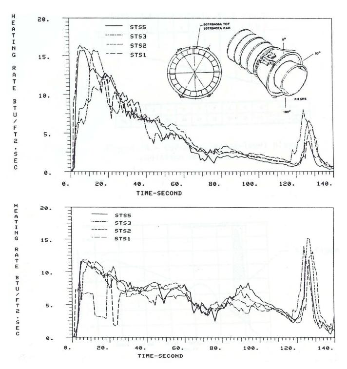
Figure 20. Right SRB Aft Skirt radiation profile. The radiation spike occurs during Tail-off at chamber pressures below 344 kPa (50 psia) and extends to vacuum conditions. Its duration coincides with prodigious solid particulate emissions from SRBs.
