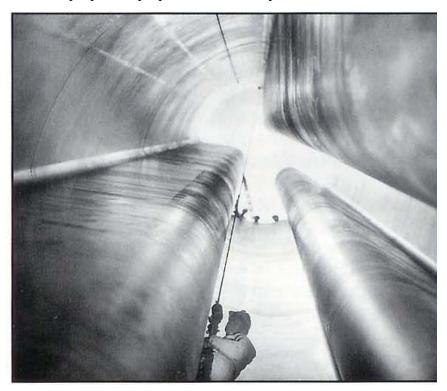
Figure 2: Interior chamber of an early 260-inch diameter SRM illustrating clearly the cast propellant grains in a 3-point configuration. This SRM was a developmental prototype of the SRBs used on the Space Shuttle. Aerojet-General Photo 2-66-SP-000.
