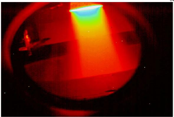
Figure 74. Main burn phase of spinning (60rpm) Star-37 SRM showing laminar plume. (Chamber pressure > 3.1 MPa (> 450 psia)).
