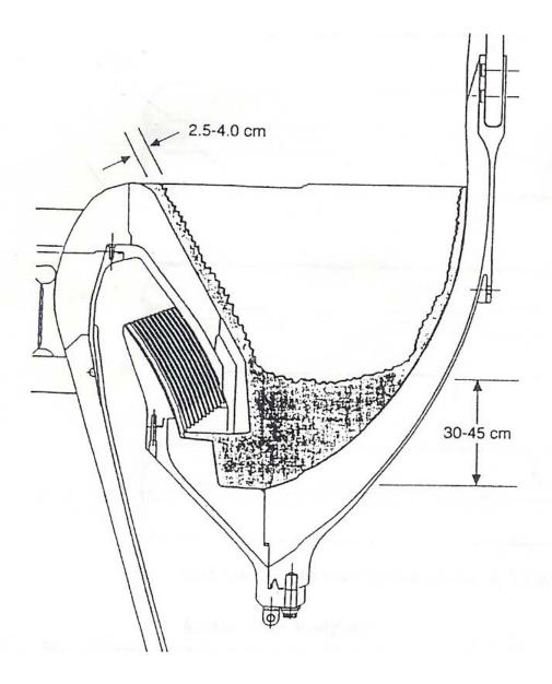
Figure 9. Cross-sectional view illustrating the solidified  $Al_2O_3$  slag generated in a SRB during a static test. The slag mass was 0.6% of the available propellant mass. A similar result is found for essentially all static SRM tests which are conducted at atmospheric pressure – and regardless of SRM orientation. (Salita 1995).
