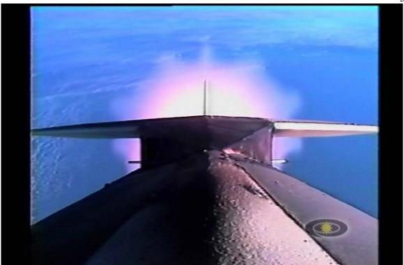
Figure 41. Tail-off -1.5 seconds. Pegaus 1<sup>st</sup> Stage SRM showing main burn phase exhaust plume devoid of any particulates of sufficient size to be individually visible. The plume consists primarily of 5-10  $\mu$ m diameter Al<sub>2</sub>O<sub>3</sub> dust.
