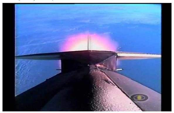
Figure 42. Tail-off -0 sec. Approximately 1.5 seconds after the previous photo, the Tail-off phase is underway. The plume is visibly smaller as the propellant is nearing exhaustion. The first large particle emission has begun (short streaks at right and left edges of plume).
