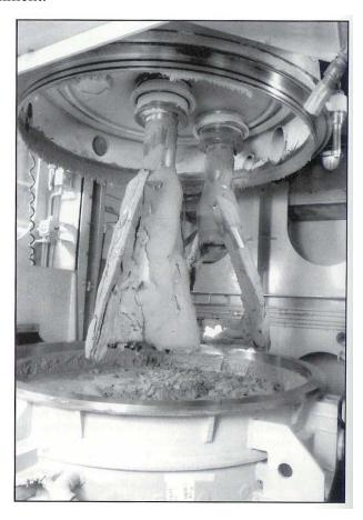
Figure 1: Solid propellant preparation. Courtesy ATK/Thiokol Photo 80110-01
