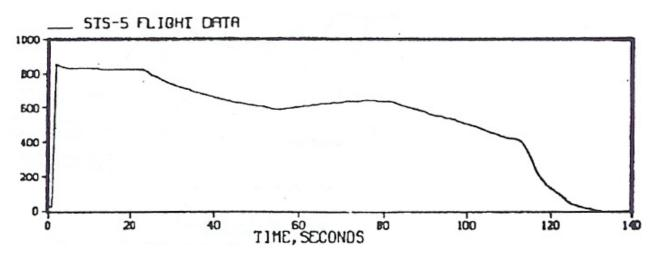
Figure 19. External Tank (ET) radiation base heating and the chamber pressure profile for comparison. The radiation spike occurs during Tail-off at chamber pressures below 344 kPa (50 psia) and extends to vacuum conditions. This behavior is consistent with slag ejection from low pressure boiling as a causative agent.
