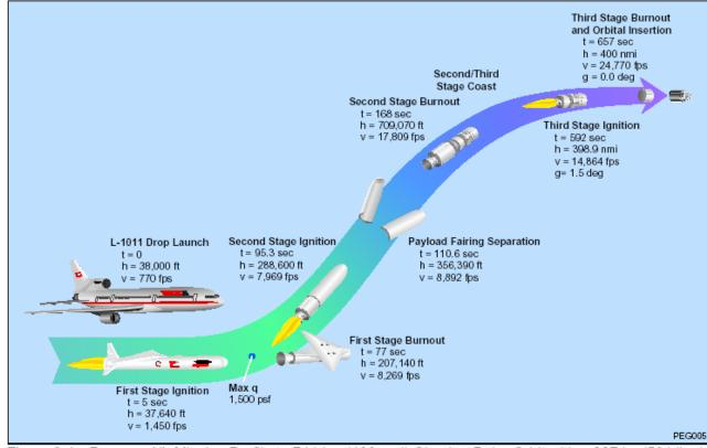
Figure 97. Flight profile for the Pegasus Launch vehicle.
