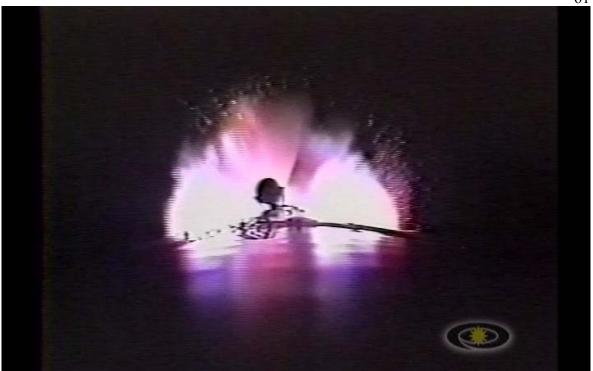
Figure 70. Night launch of a Delta II (July 16, 2000 GPS IIR-5). This image was acquired during Air-lit SRM Tail-off at 5.5 seconds prior to separation. Particle emissions are readily evident and persist until separation. Note the expanded plume under high vacuum.
