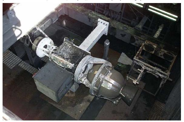
Figure 73. Star-37 SRM with 1045 kg of propellant shown loaded into the J-6 test cell. Various sensors (eg. optical and IR imagers, pressure sensors (cell and chamber)) surround the motor.
