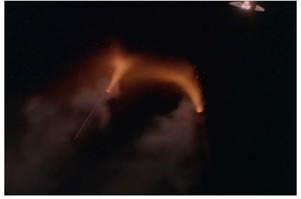
Figure 31. Separation +22.5 seconds. Chamber pressure < 6.9 kPA (< 1 psia). Numerous Tail-off ejecta are clearly resolved as the plume brightness fades.
