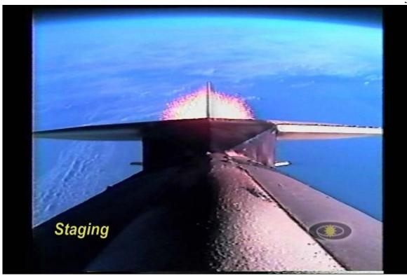
Figure 45. Tail-off +11.5 sec. A burst of several thousand large particles is emitted. Sizes are estimated to be of order 1 cm diameter.
