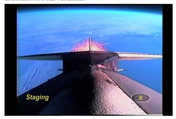
Figure 46. Tail-off +15.5 sec. Bulk large particle emission continues for approximately four seconds before diminishing to a sporadic rate.
