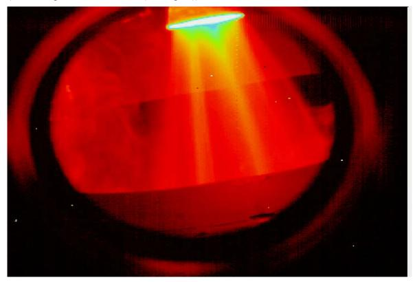
Figure 75. Onset of Tail-off in Star-37 static vacuum test. (Chamber pressure < 344 kPa (< 50 psia)).
