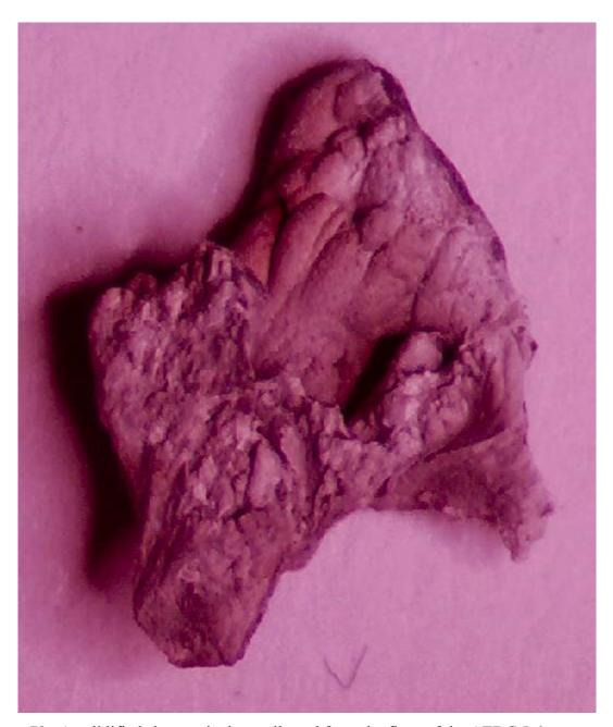
Figure 79. A solidified slag particulate collected from the floor of the AEDC J-6 test chamber after the Star-37 static vacuum test. SEM microscopy (Bernhard 2004) shows that it is composed of  $Al_2O_3$ . Its flattened appearance may due to impact with the test chamber floor while still in a molten state.
