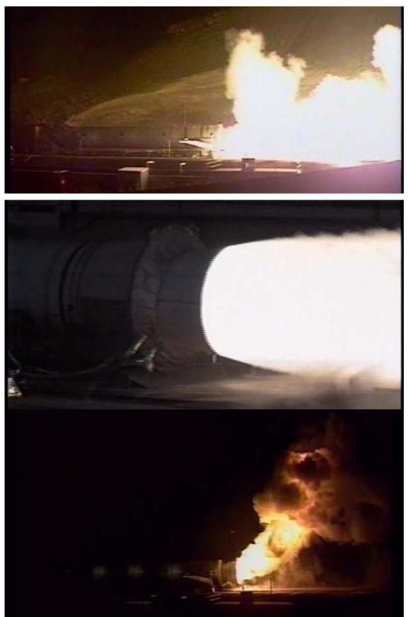
Figure 12. Optical imagery of Static SRB test. Slag expulsion is not evident at Tail-off (last frame). (Thiokol Photos).
