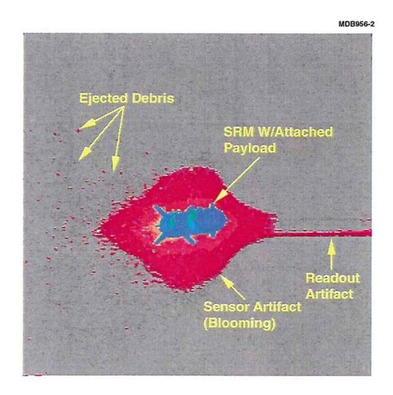
Figure 80. Mid-Wave IR (MWIR 3-5  $\mu$ m) image of a rocket body and associated SRM late stage Tail-off ejecta. This image was acquired by a Fly-Away-Sensor Package (FASP) between 40 seconds and 100 after the beginning of Tail-off. (Berstein and Sheeks 1997).
