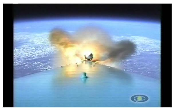
Figure 62. Air-lit SRM boosters exhibit comparable behavior to ground-lit motors. During the main burn phase (shown here), no large particulates are evident. Figs. 62-65: April 7, 2001 Delta II Odyssey air-lit SRM booster on 1<sup>st</sup> stage.
