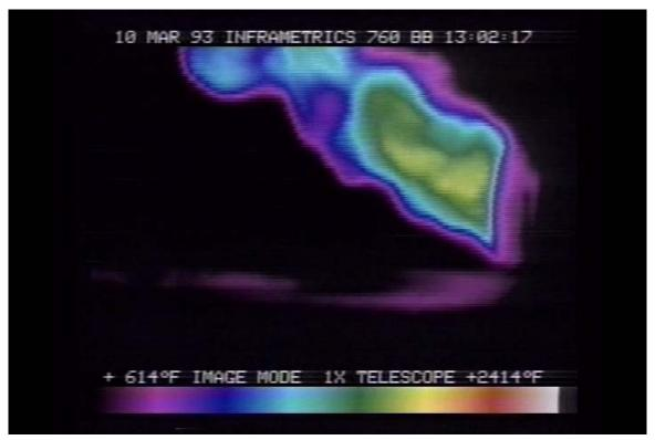
Figure 17. SRB Static test (non-vacuum) – Late Tail-off. Chamber pressures are near ambient atmospheric. No solid particulate emissions are discernable. (Thiokol photo).
