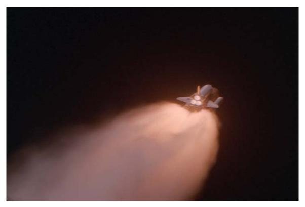
Figure 24. STS-101 Time Sequence. Separation -4.0 seconds; Chamber pressure  $\sim$ 275 kPa ( $\sim$ 40 psia). No Tail-off ejecta present.
