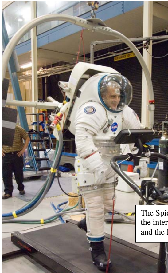
Figure 2: MK Suit and Spider-Gimbal System Test Set Up
