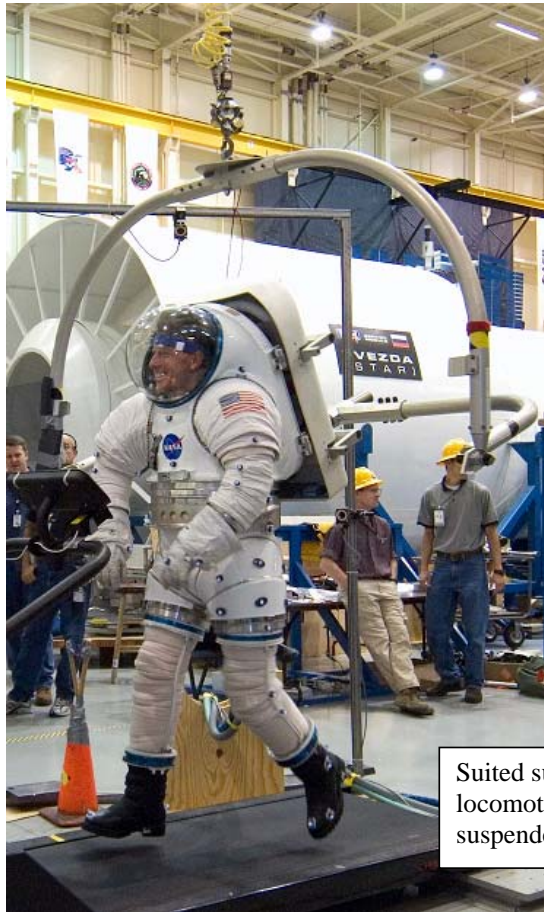
Figure 4: Subject Performing 10 km Translation in MK III Suit in Lunar Gravity
