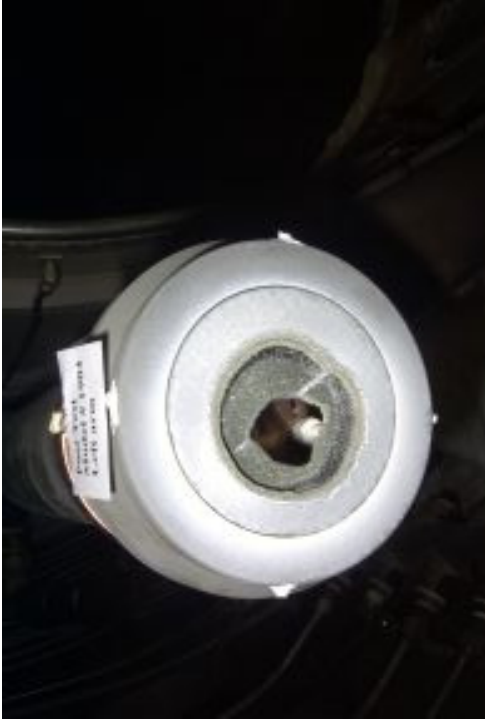
Front-side Post-Test View of 0.030" Dia. Slot
