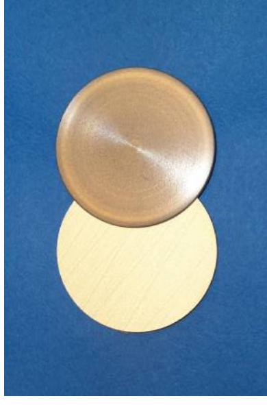
Ceramic TC Sputtering Targets fabricated by the CWRU & NASA GRC Ceramics Branch
