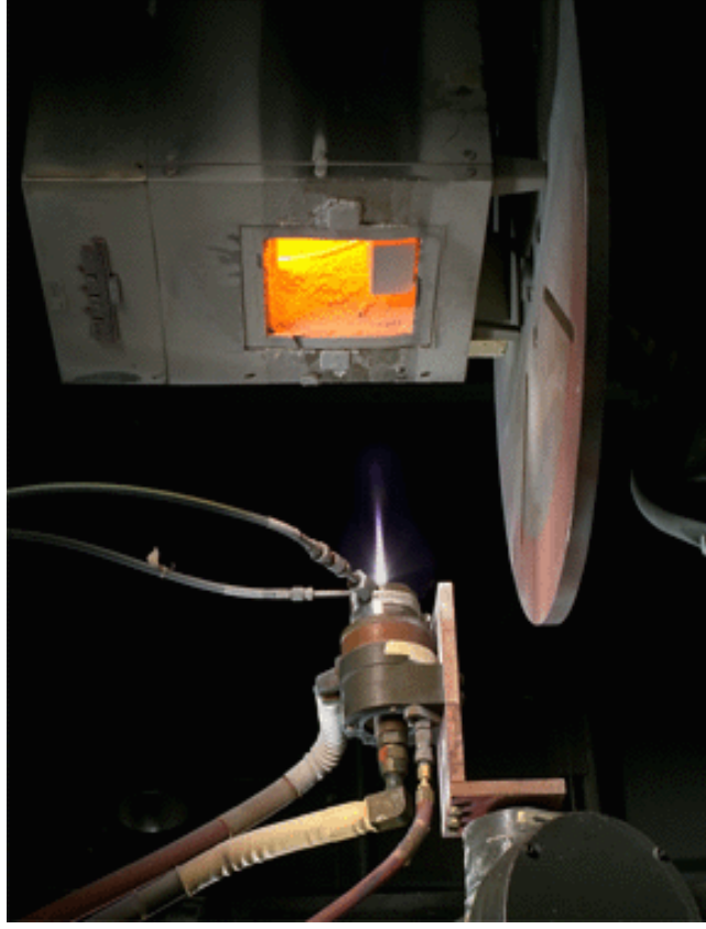
Plasma-spray processing of Environmental barrier coatings for various components
