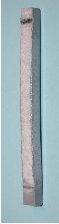
Composite EBC coated AS 800 Si 3 N 4 rupture testing (completed 691 hrs 2500°F 1371°C, 250 MPa without failure)
