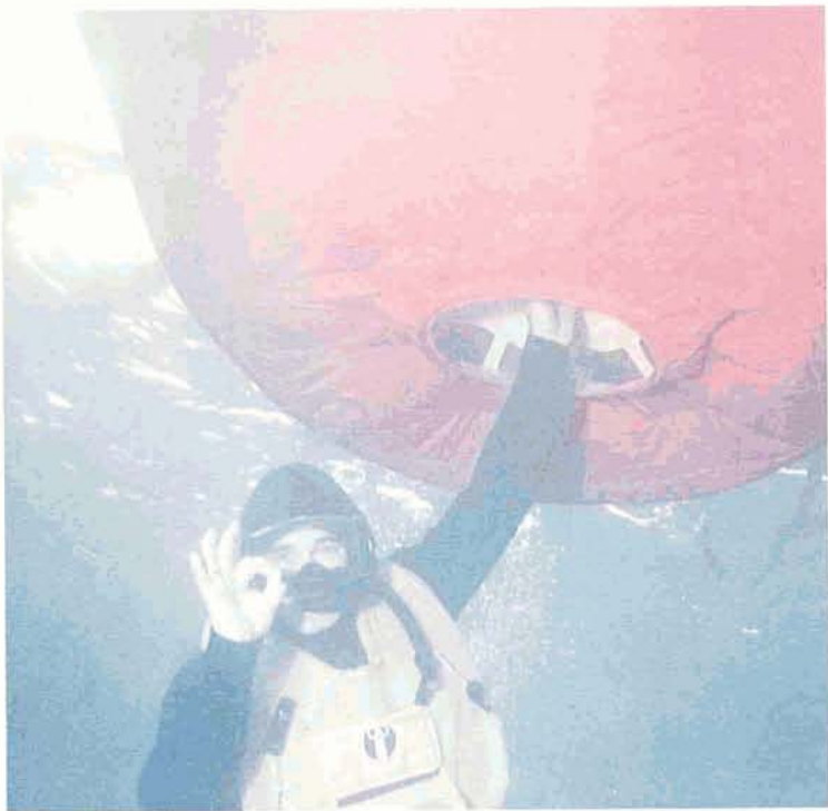
In this underwater view, the diver is examining the "flapper valve" of the Givens Buoy Raft. The valve admits water to the large hemispheric ballast chamber, key to the raft's exceptional stability.
