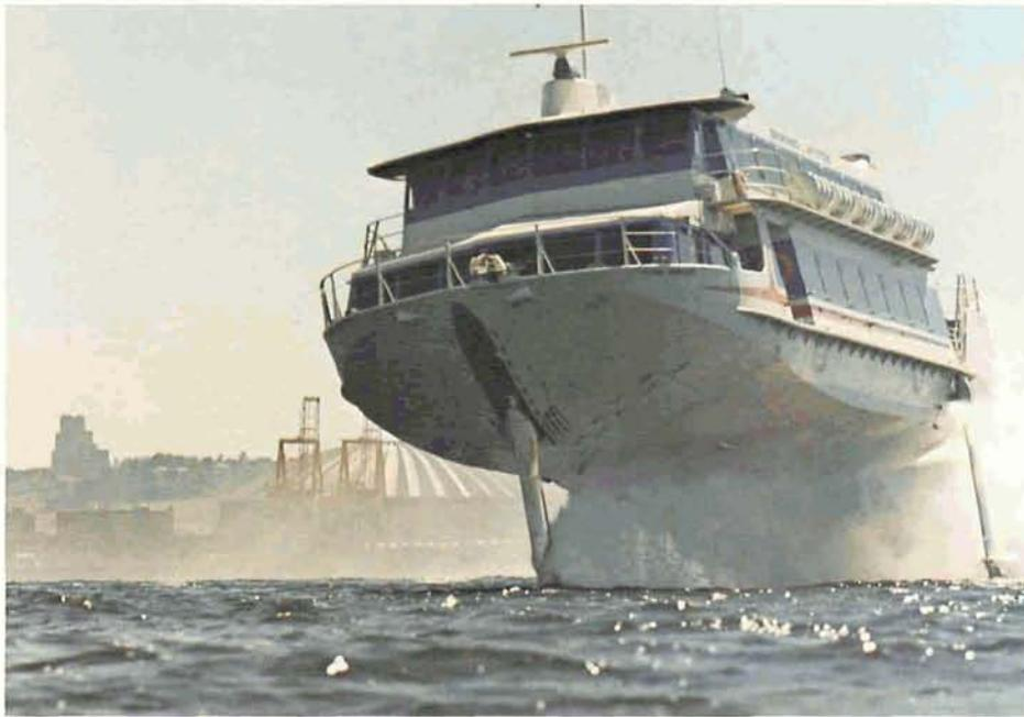
*This photo of a Boeing Jetfoil shows how the hydrofoils lift the vessel's hull well above the surface, enabling the Jetfoil to cruise at 45 knots because of minimal friction between hull and water.*
