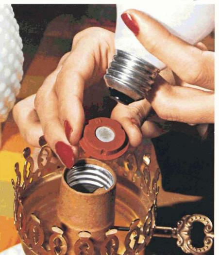
Bulb-Miser You probably have noticed that most light bulbs fail when you flick on the light switch. That's because the initial impact of the full current is too much for the cold filament. A new product called the Bulb-Miser\* provides the answer to a problem for large quantity bulb users. It acts as a thermal shock absorber and lets the filament heat up slowly to prevent burnout. The result: an average increase in bulb life of 300 percent.
