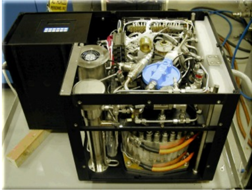
Figure 3.5.—Treadwell Corporation PEM Electrolyzer Unit.
