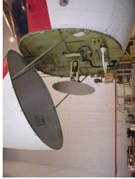
Installation of the E-Turb radar, a modified radar unit that can detect turbulence associated with thunderstorms by measuring the motions of the moisture in the air.
