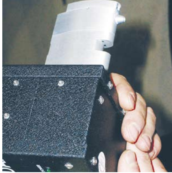
Shown here is the TAMDAR instrument, a tiny sensor flown on commuter airliners to gather weather information.
