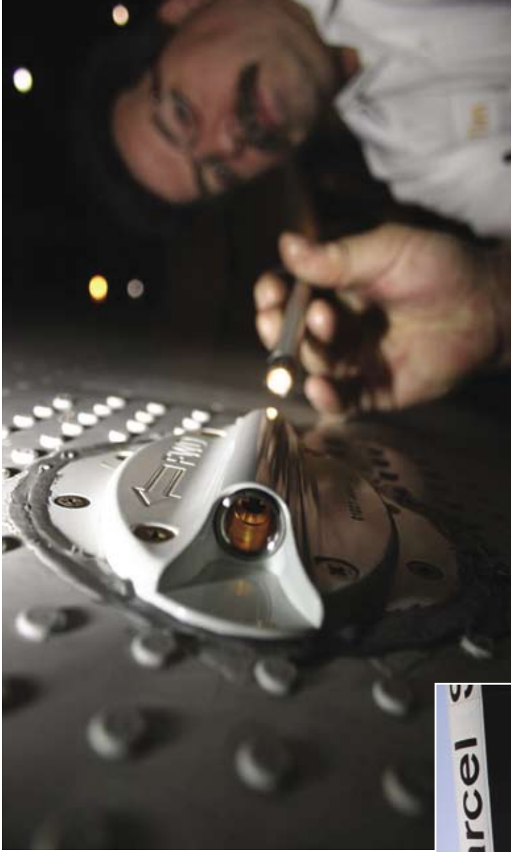
The air-sampling device was built to be mounted onto the side of a plane. Its aerodynamic design removes ice crystals, particles, rain, and other distractions to improve the sensitivity of the air measurement.
