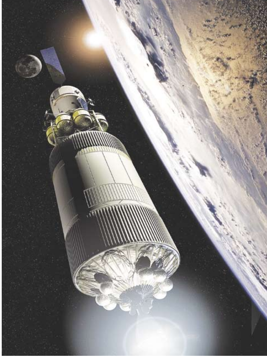
A rocket fires for translunar injection, carrying the Crew Exploration Vehicle and lunar lander toward the Moon.
