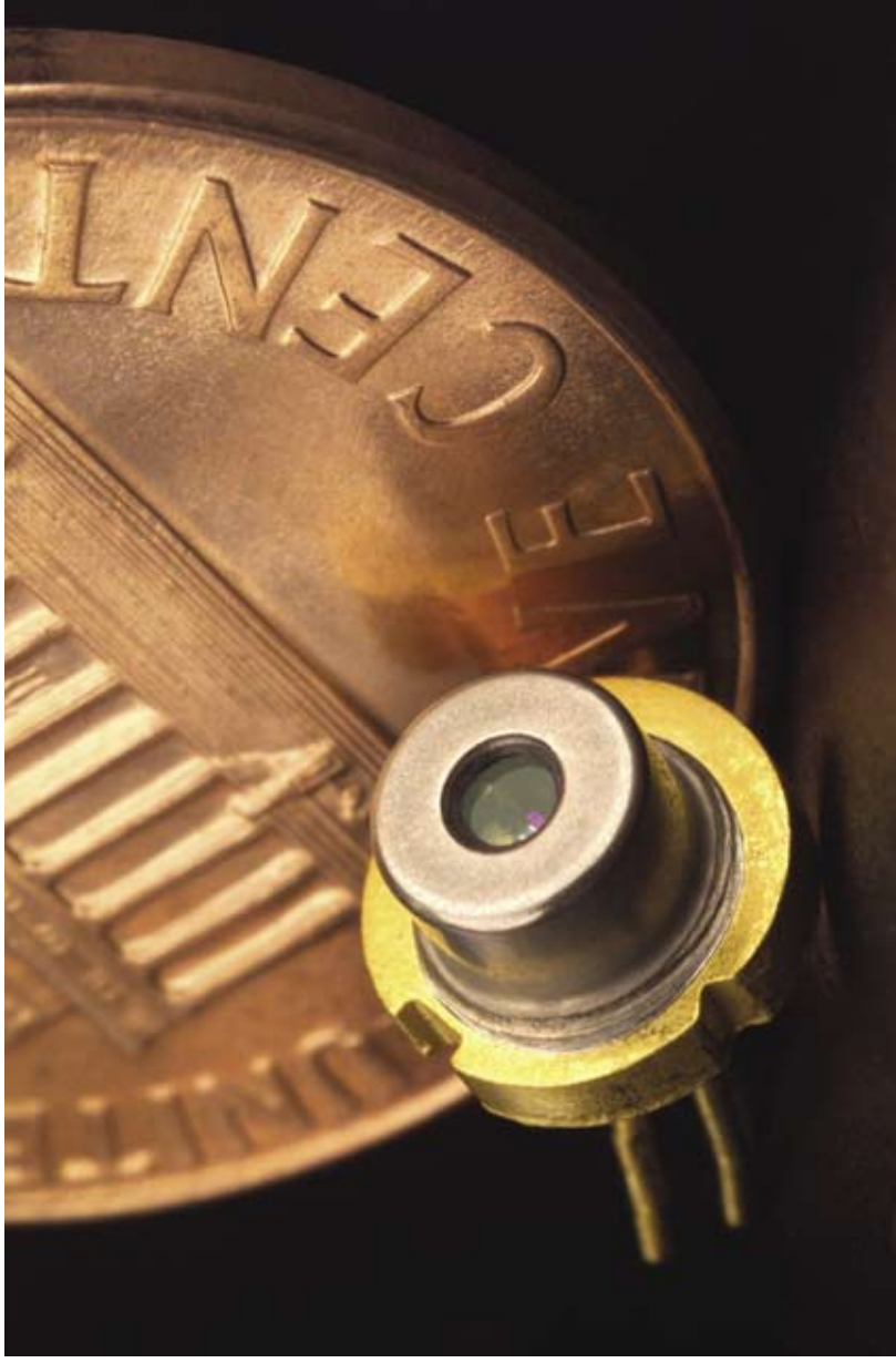
Miniaturized tunable diode laser packaging for sensing and measuring atmospheric water vapor.
