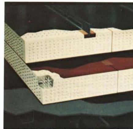
layers of a new type of 3D designed specifically for the special needs of LNG containment. Above is a cutaway of the combined Invar-3D system. The top layer of Invar is the primary barrier, in physical contact with the LNG. The secondary barrier, shown in white, consists of two four-inch layers of 3D separated by a fiberglass liner. The Gaz-Transport/McDonnell Douglas system offers reduced boiloff, high strength, low cost and long durability.
