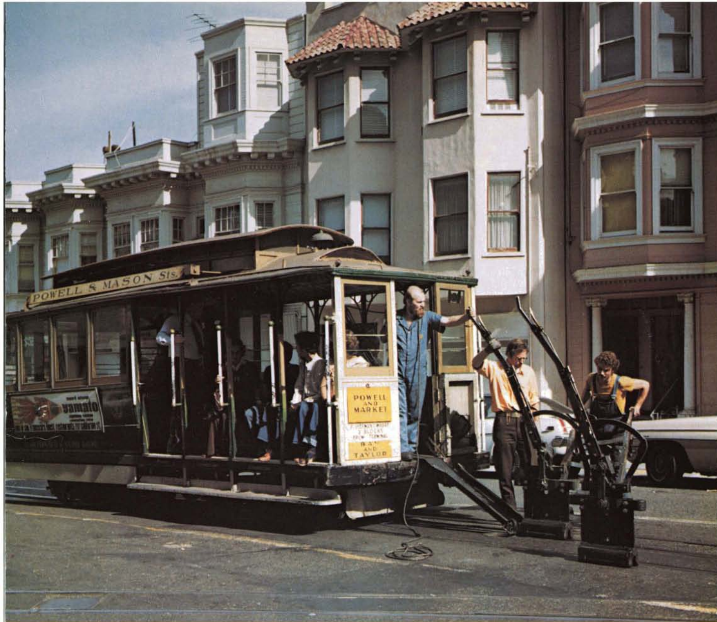
In the photo, technicians of the San Francisco Municipal Railway—"Muni"—are exchanging a cable car's grip, used by the operator, or "grip-man," to clasp the moving cable which pulls the car along. NASA's Ames Research Center is improving the grip design.
