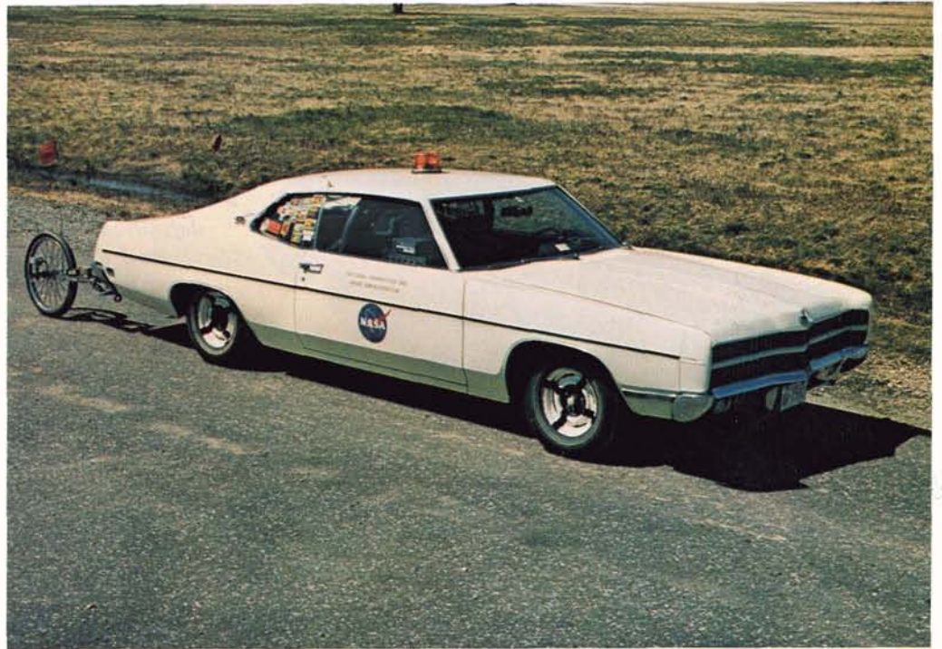
A NASA-developed five-wheeled vehicle serves as a mobile laboratory for testing roadway skid resistance. It does a job comparable to more expensive test vehicles, but at a fraction of the cost. Cost is a big factor to many communities, which need skid resistance data for improving road surfaces but can't afford highly expensive skid trailers and their elaborate instrumentation.
