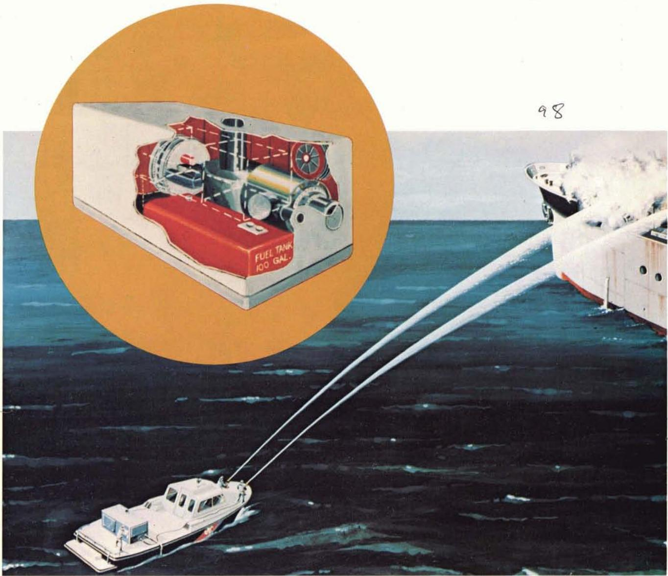
which delivers 2,000 gallons of sea water per minute, a quick starting gas turbine, hose, monitors, nozzles, protective suits, and other equipment.
