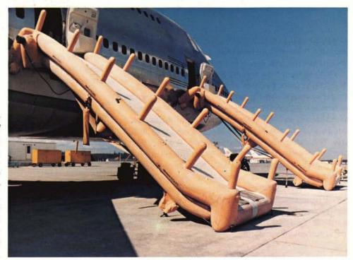
These Boeing 747 escape chutes, for rapid evacuation of passengers in a ground emergency, are inflated by filament-wound pressure vessels, 60 percent lighter than earlier inflation cylinders. Changeover to the new bottles, spinoffs from rocket motor casing technology, saves 200 pounds per airplane.
