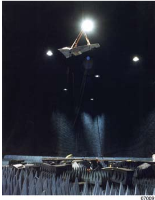
Figure 16. Antenna pattern testing in the Benefield Anechoic Facility at Edwards Air Force Base.
