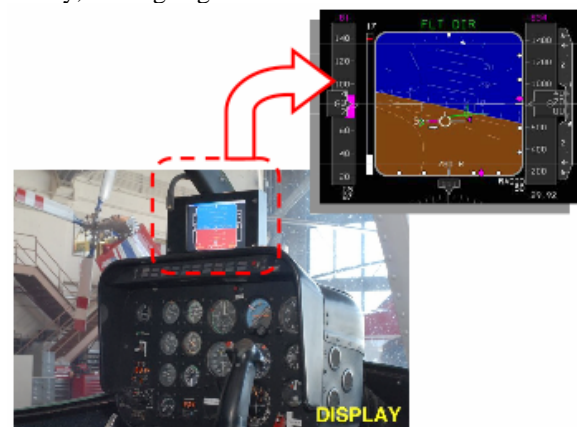
Figure 8 The PPGD Display Mounted Over the Instrument Panel of the Bell 206B Helicopter
