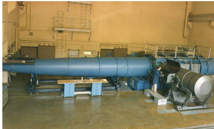
Figure 2. AEDC Hypervelocity Wind Tunnel No. 9 Test Cell and Mach 10 Nozzle
