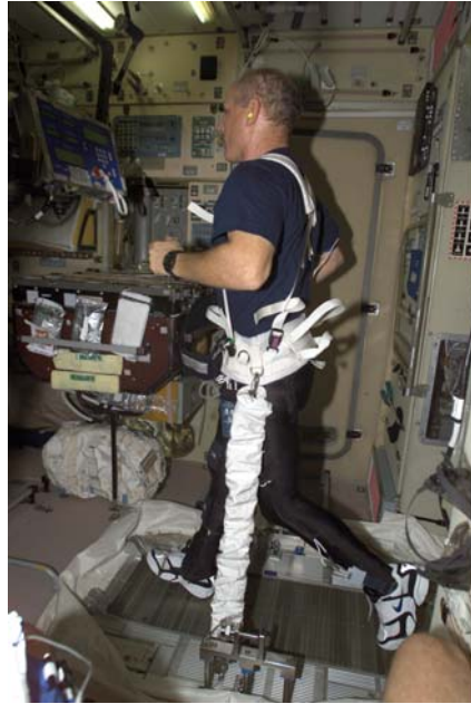
Figure 1. Astronaut exercising on a treadmill onboard the International Space Station. The astronaut is wearing a harness around his waist and shoulders and is connected to the treadmill via elastic bungee cords (vertical attachment between the harness and treadmill).
