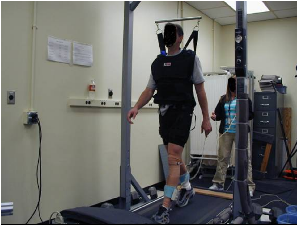
Figure 3. Typical data collection with the H/P Cosmos Airwalk Unweighting System and Weighted X-Vest.
