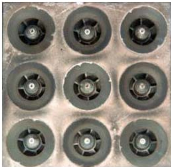
Figure 1: 9-element fuel injector module
