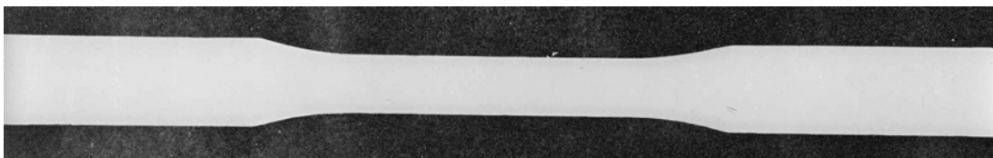
Figure 163. Representative LDPE tensile specimen.
