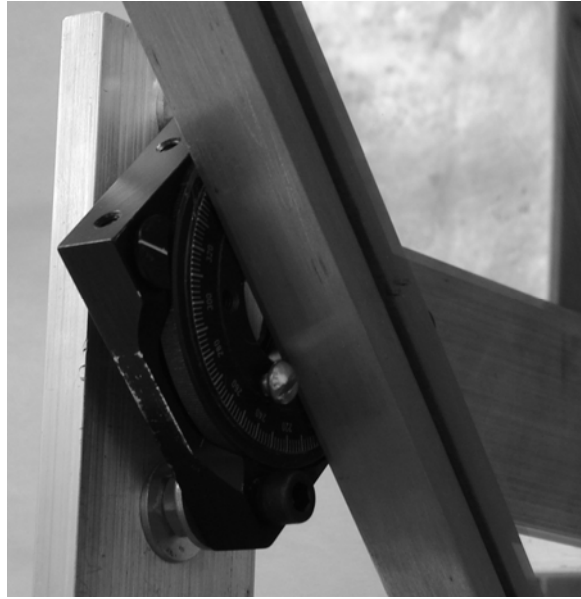
Figure 122. Close-up photograph of the top rotating base on the 45° mirror holder.
