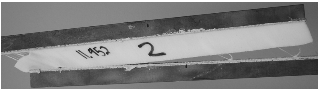
Figure 72. Delamination failure of a 0.62 stitch/cm 2 Voltek PE core shear specimen.
