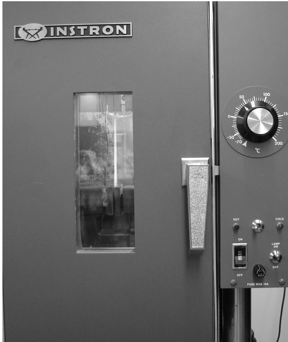
Figure 166. Tensile specimen within a circulating convection oven.
