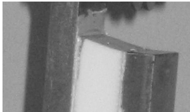
Figure 62. Delamination in a non-stitched PE core shear specimen.
