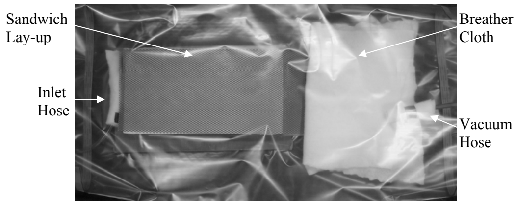
Figure 4. Vacuum bag and hose sealed with vacuum tape.
