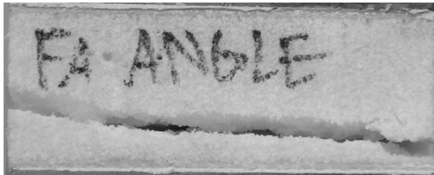
Figure 49. Core cracking in angle stitched PET specimen following vertical stitch failure.
