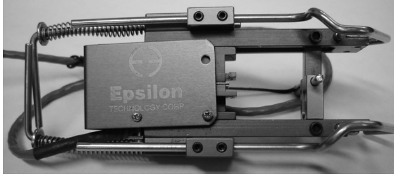
Figure 164. Extensometer used for displacement measurements.
