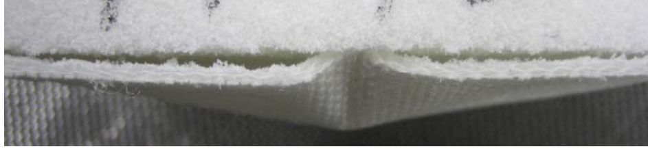
Figure 84. Lower facesheet wrinkling following partial separation from the lower core.
