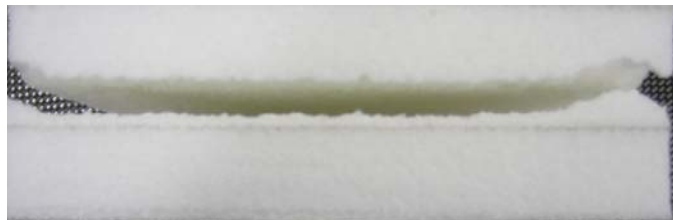
Figure 83. Separation of interior laminate from the upper core following failure
