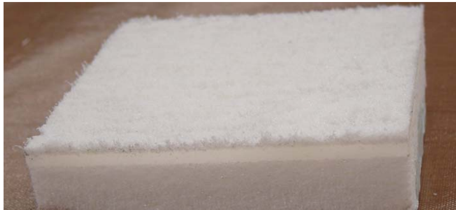
Figure 54. Representative PET/Surlyn bond failure.
