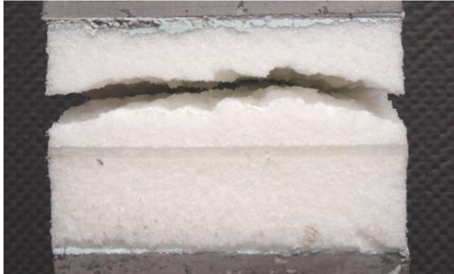
Figure 53. Representative PET foam failure.
