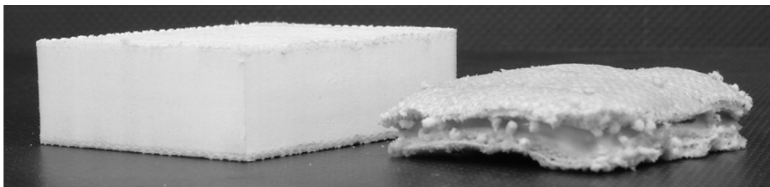
Figure 129. Representative PE/Spectra specimen before and after environmental testing.
