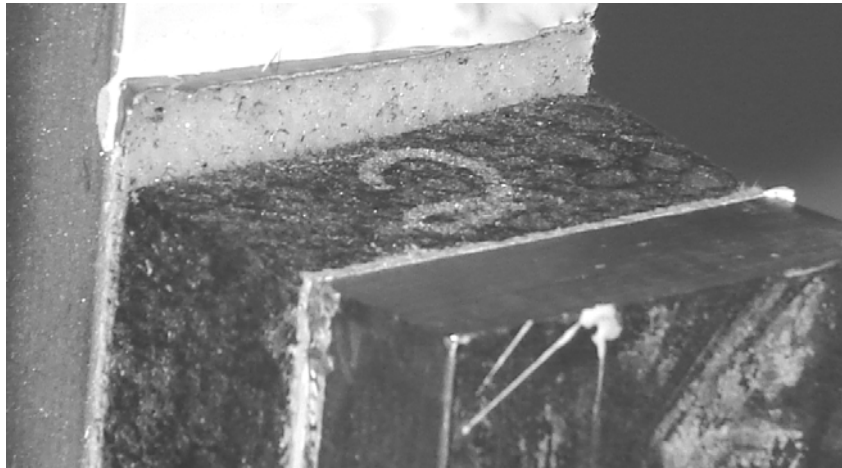
Figure 66. Initiation of delamination at the leading edge of a 0.16 stitch/cm 2 PP specimen
