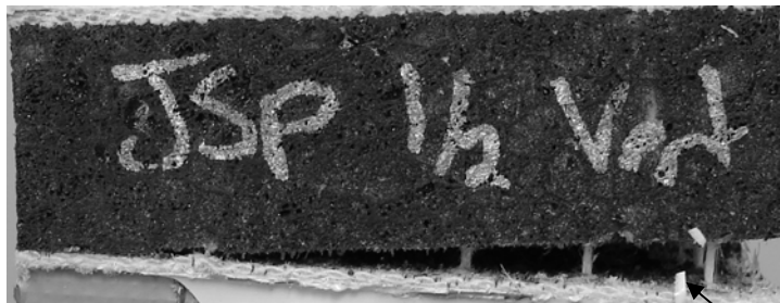
b. Failure of first stitch row.
