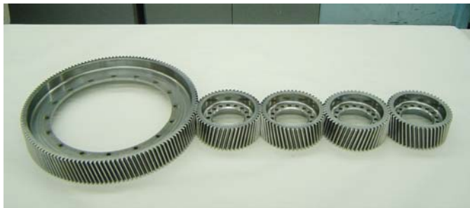
Figure 8.—Entire gear train after superfinishing.
