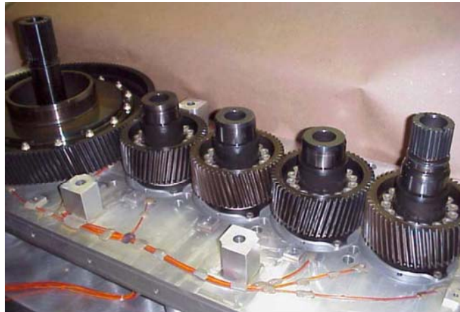
Figure 6.—Baseline gear train installed in half of the test gearbox.
