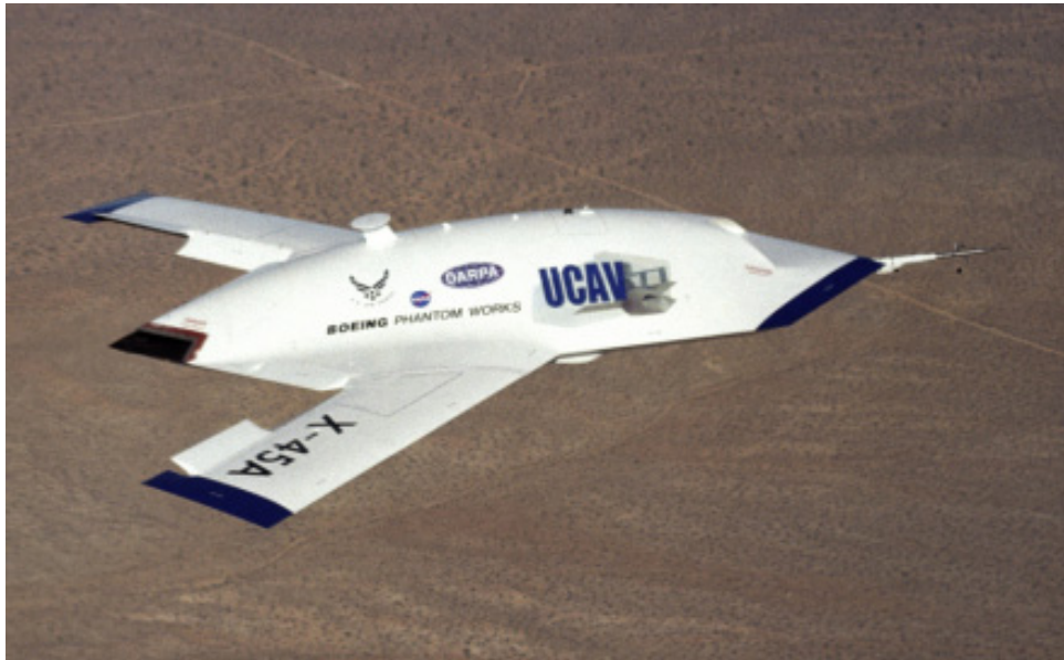
Figure 1.3: Figure 3. The X-45A Unmanned Combat Air Vehicle in flight over the Mojave Desert.
