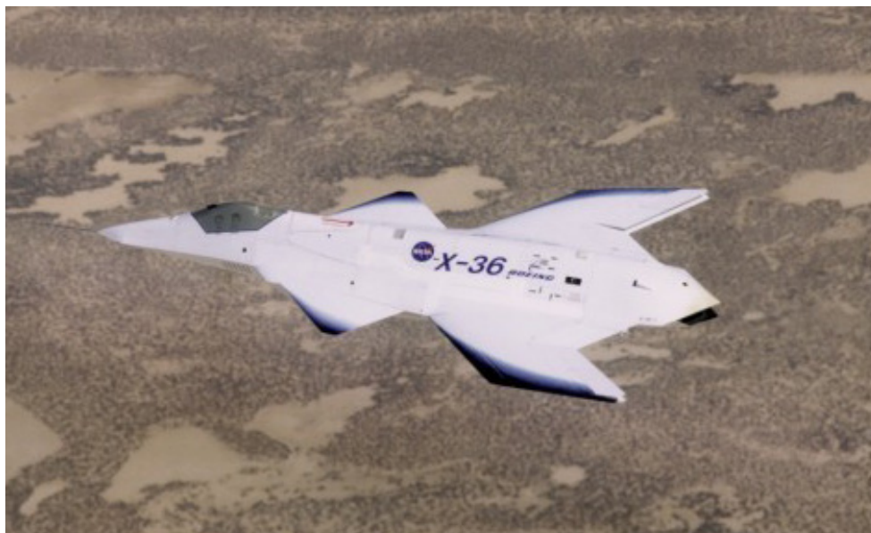
Figure 1.1: The X-36 Tailless Fighter Agility Research Aircraft in flight over the Mojave Desert.
