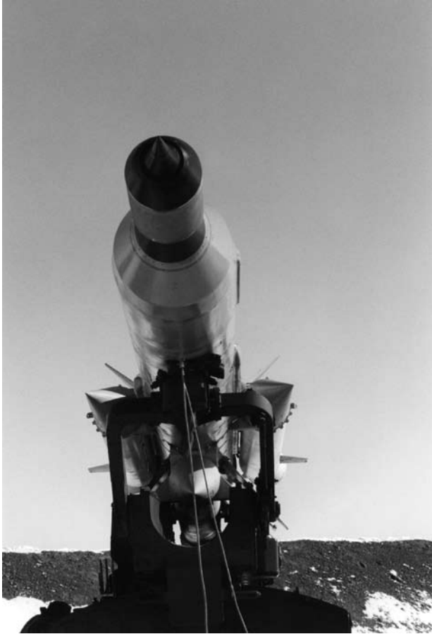
The CIAM Mach 6.5, model 58L, flight test scramjet.
