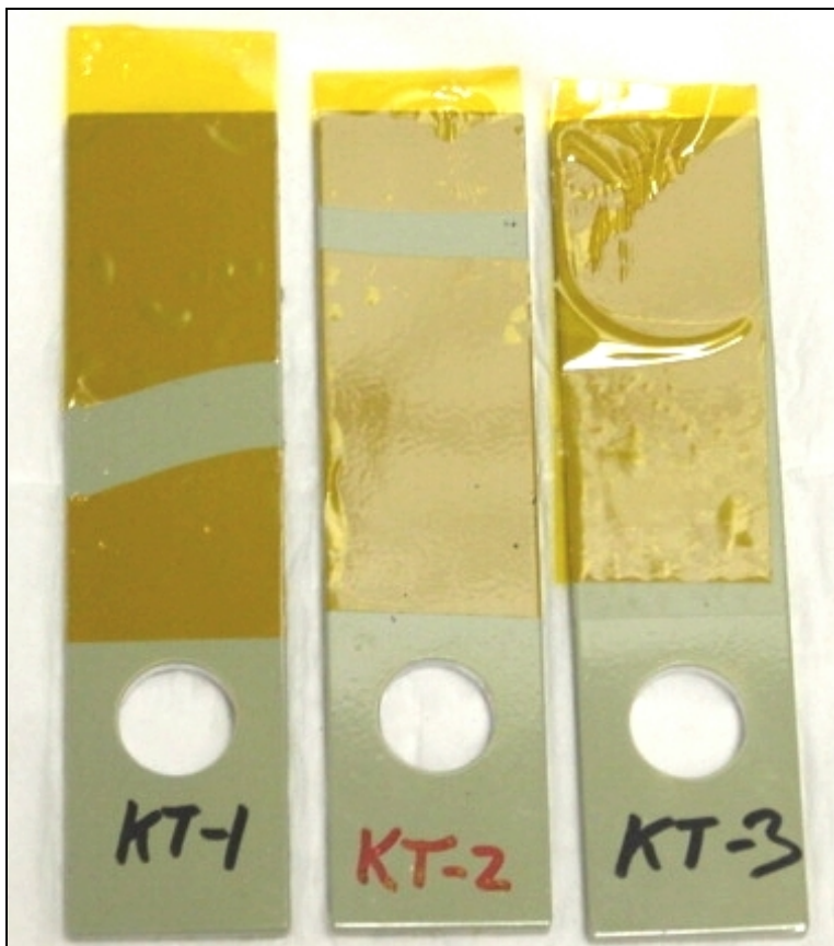
Figure 18. Failed Kapton tape and adhesive resulting from uncoated DLS testing.
