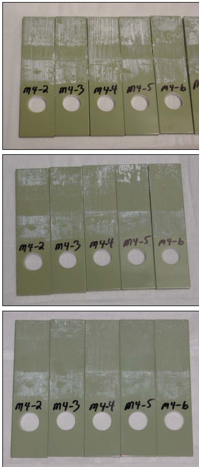
Figure 17. M4 coupons after one (top), two (middle), and three (bottom) test cycles.
