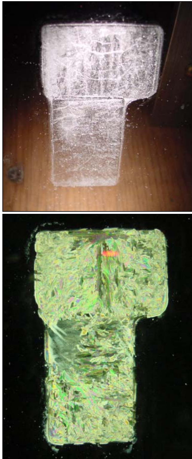
Figure 29. Ice samples from two sides of mold M4-2(5) with point backlighting (top) and cross-polarized light (bottom).
