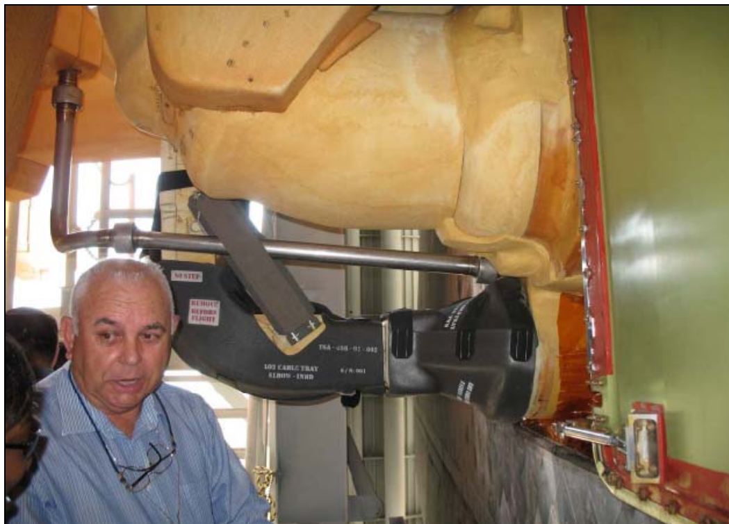
Figure 4. STS-115 LO 2 umbilical area access from the platform on the launch pad, 23 August 2006 preflight inspection.
