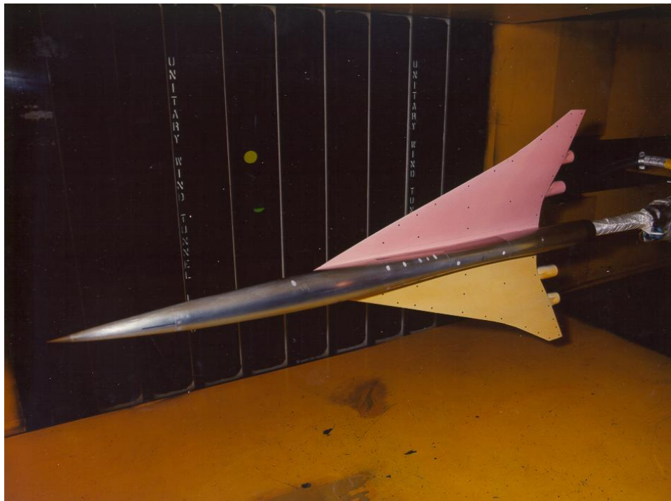
Figure 17. Arrow wing model installed in UPWT Test Section 1 with PSP (upper wing) and TSP (lower wing) coatings.
