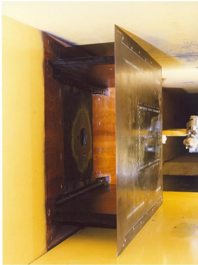
Figure 58. Flutter panel fixture mounted to the side wall in UPWT Test Section 1 (view looking downstream).
