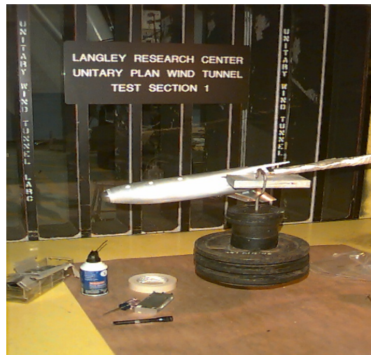
Figure 10. Check load application to instrumented canted fin using weight pan hanger.
