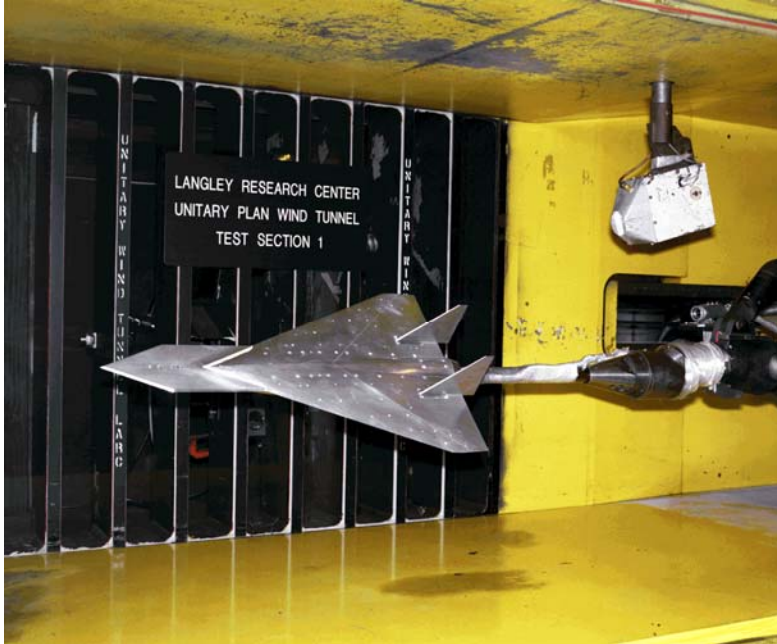
Figure 5. Test-ready general research fighter model.
