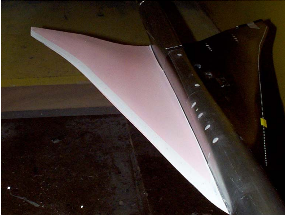
Figure 39. Close-up view of an arrow wing model with PSP coating (the leading-edge region is buffed for boundary layer transition trip dot application).
