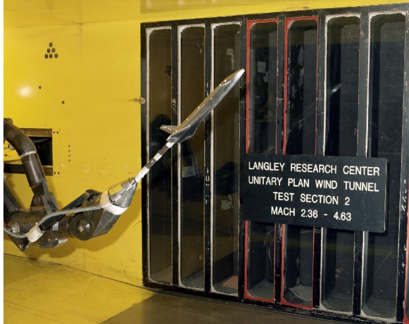
Figure 70. 1.75%-scale glideback booster model installed on the high angle-of-attack apparatus in UPWT Test Section 2.
