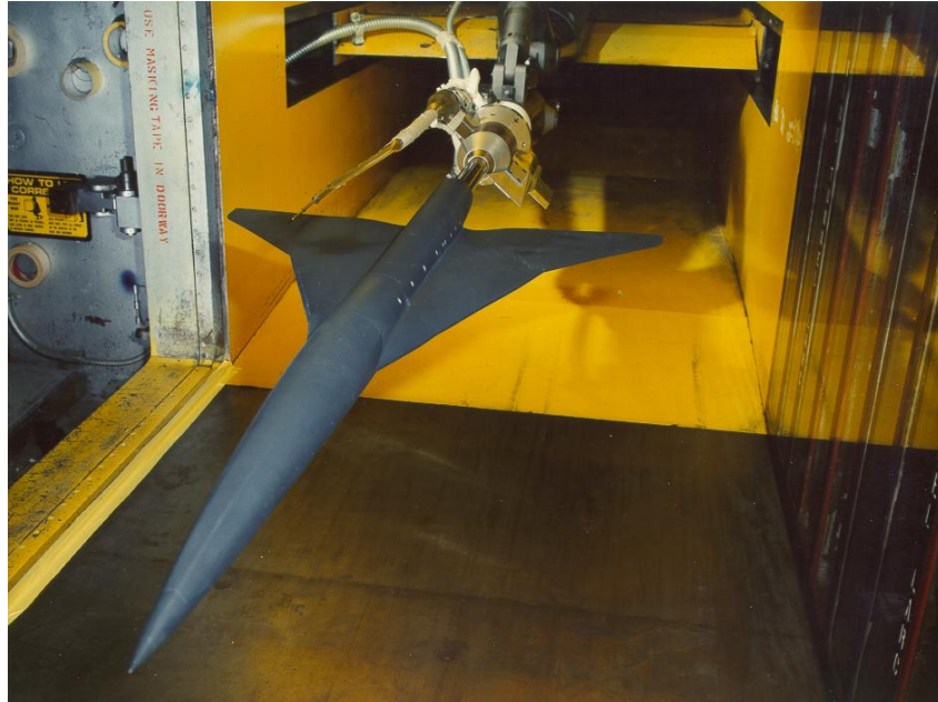
Figure 64. Supersonic transport model with flow field survey apparatus in UPWT Test Section 1.
