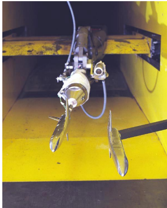
Figure 74. Simulated spatial positioning in a stage separation trajectory.
