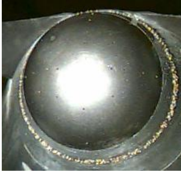
Figure 12. Close-up photograph of pressure-instrumented nose cap for FADS calibration on a 2%-scale X-33 model in UPWT.
