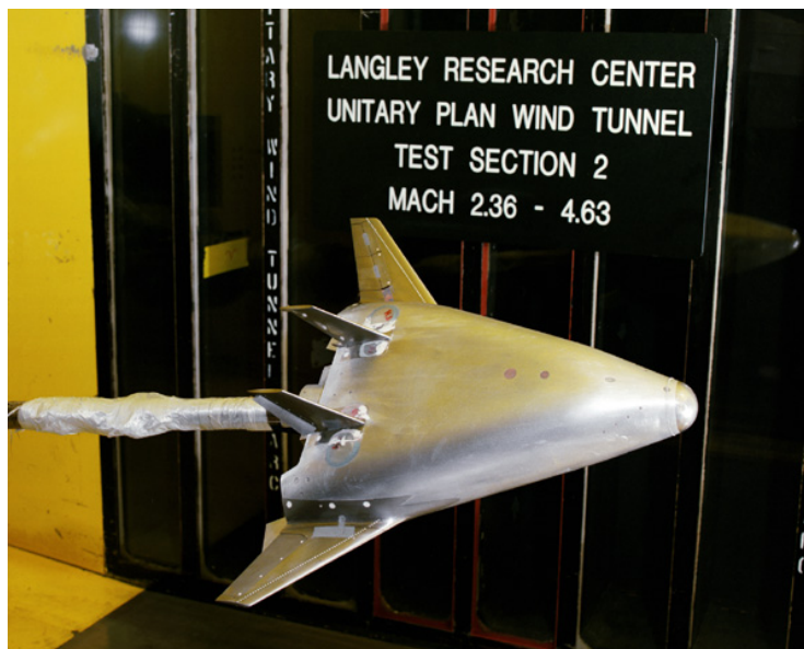
Figure 8. 2%-scale X-33 loads model installed in UPWT Test Section 2.
