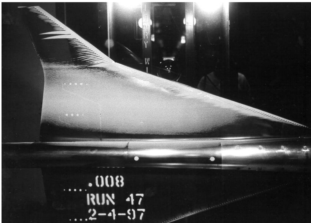
Figure 42. Surface sublimation pattern on a slender wing at Mach = 2.4 in UPWT Test Section 2.
