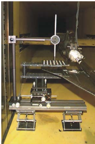
Figure 25. Video model deformation system calibration setup in UPWT Test Section 1.
