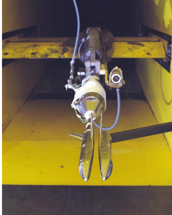
Figure 73. Simulated captive bimese arrangement using the UPWT stage separation setup.
