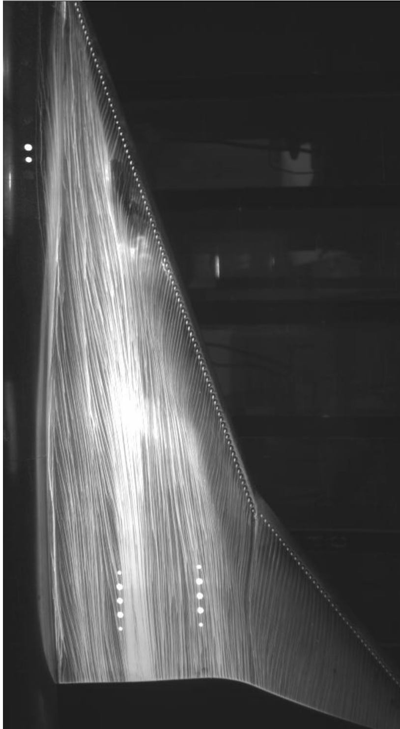
Figure 43. UV oil pattern on a slender wing model at Mach = 2.4 and \alpha = 4.5 degrees in UPWT Test Section 2.
