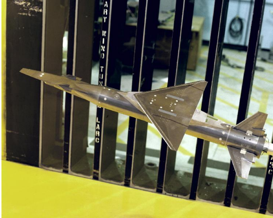
Figure 71. 6%-scale Hyper-X stack configuration installed in UPWT Test Section 1.
