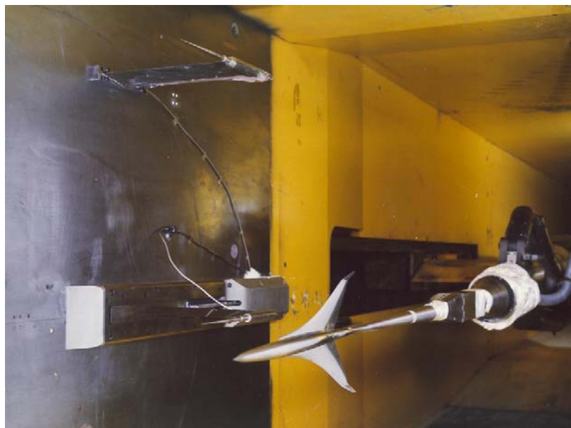
Figure 59. Sonic boom pressure measurement setup in UPWT Test Section 1.
