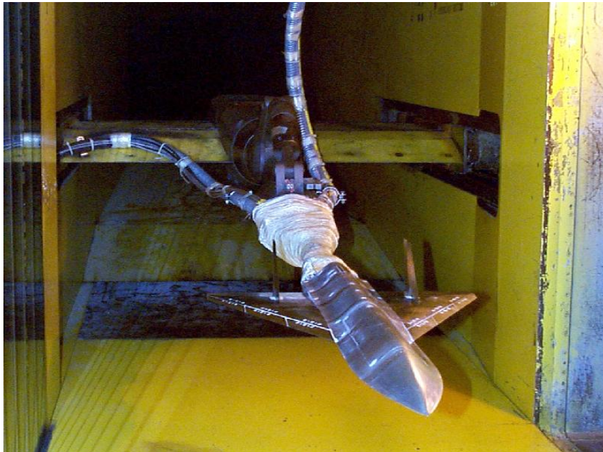
Figure 13. MTVI model configured for dedicated surface static pressure measurements in UPWT Test Section 1.
