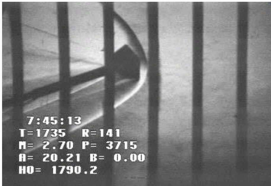
Figure 78. Schlieren flow visualization images of a Mars lander model at Mach = 2.7 in UPWT Test Section 2.
