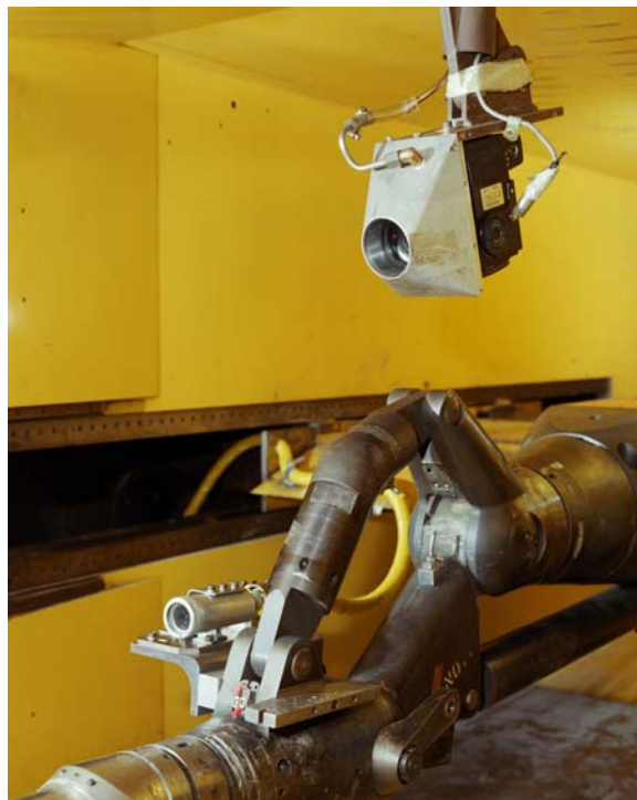
Figure 53. Still and video camera installation for vapor screen flow visualization in UPWT Test Section 1.
