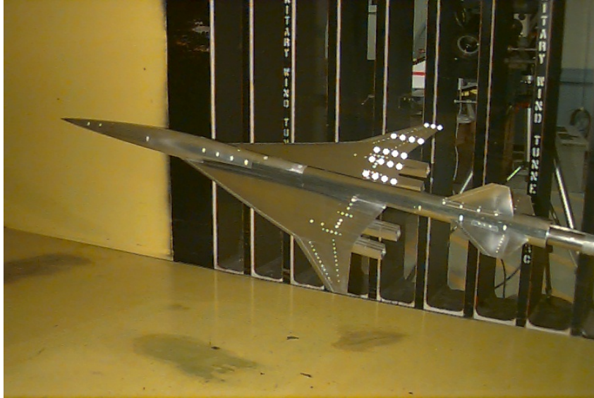
Figure 26. Supersonic transport model installed in UPWT Test Section 1 for wing deformation measurements.
