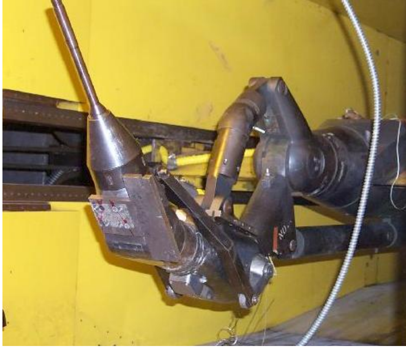
Figure 69. UPWT high angle-of-attack apparatus installed in Test Section 1. (Calibration plate shown on lower surface is installed for wind-off calibrations only.)
