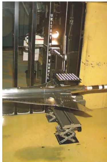
Figure 25. Video model deformation system calibration setup in UPWT Test Section 1.
